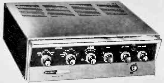
Heathkit 50-watt amplifier ($85) is kit model No. AAW-100; response is 30 to 15,000 at full output.
