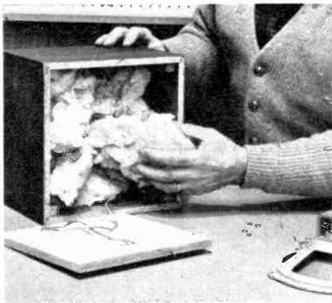
BE CAREFUL not to overdamp the speaker by packing in too much damping material.
