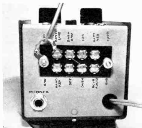
Rear terminal board takes connections to transmitter for keying, to receiver for optional monitoring and has a jack for a conventional key.
