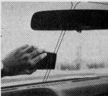
One of the many uses for your calculator other than calculating. Here it is being used to check a windshield antenna.
