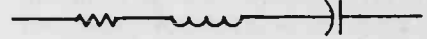
Fig. 6. Diagram is a typical equivalent circuit for a crystal. As resistance is lowered to near zero; crystal efficiency increases. In use, the crystal holder and external circuit add some capacitance across the entire circuit.
