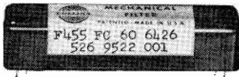
Fig. 7. This is the type of filter used to remove the unwanted sideband from the RF output signal.
