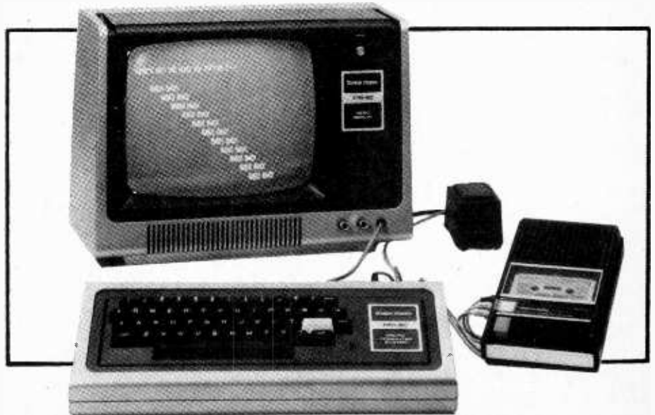
Complete computer systems for the home can be bought off the shelf from various companies. Shown here is the Radio Shack TRS-80 micro computer system. It features an ASCII keyboard-equipped computer that can be mated to numerous peripherals.
