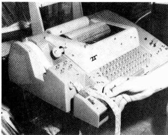
The punch/reader of an ASR-type teletypewriter is one of the more common systems. It's very easy to use; just push a button to transmit a signal from the computer and it will punch or read a tape or do both.
