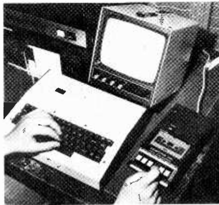
You don't need a special interface for the CC8 "Computer Aid" recorder.
