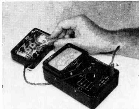
F The completed unit with 40 ua meter movement being used to check pocket-sized transistor receiver.
