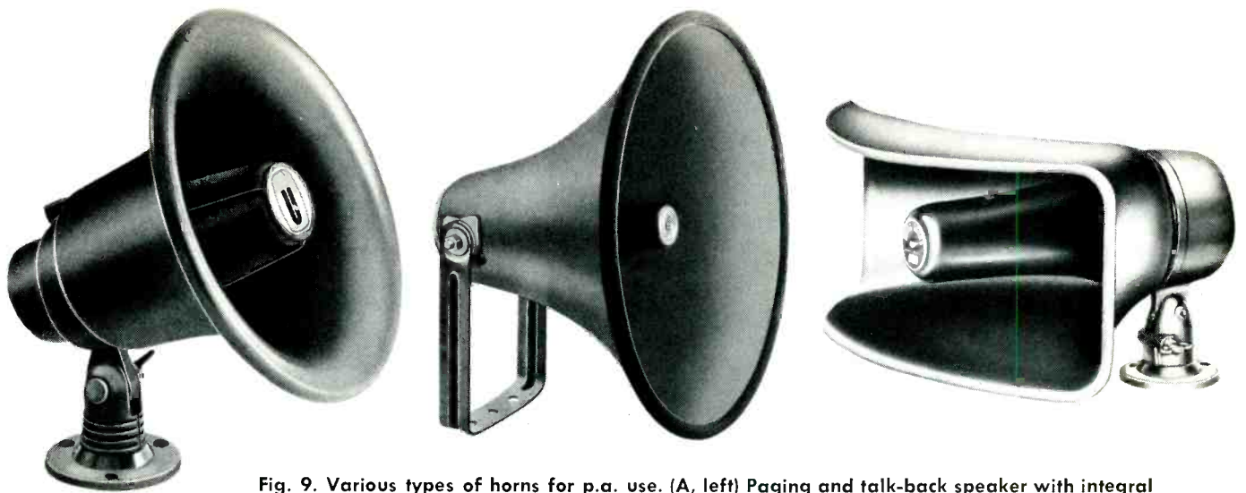
Fig. 9. Various types of horns for p.a. use. (A, left) Paging and talk-back speaker with integral driver unit, University MIL-A; (B, center) long-throw projector with provision for screw-on driver unit, University GH; (C, right) contoured horn for wide-angle distribution, Atlas CJ-30B.
