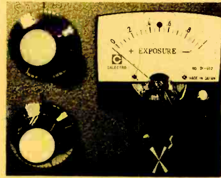
Close-up of meter face showing a small scale-illumination lamp in lower right corner. This lamp should not be operated at full voltage to avoid fogging the film.
