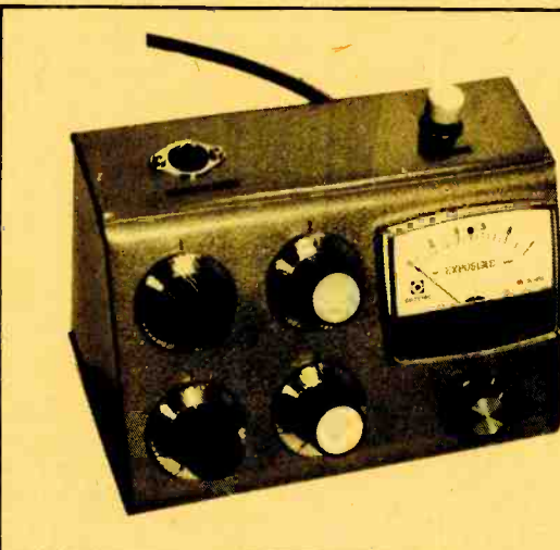
To avoid upsetting a control setting while groping for the on-off switch in the dark-room, mount switch S2 as far as possible from the controls.
