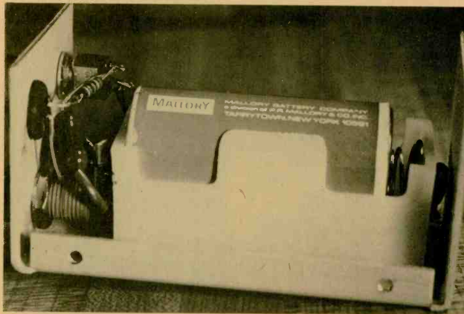
Fig. 3. The compact construction of the calibrator is seen here. We wired all components to the terminals of the banana jacks first, and then bolted in the battery holder to the bottom of the chassis to allow working room for assembly. You may choose to utilize either perfboard or even a printed circuit board for your model. This will allow you to mount it directly inside the cabinet of whatever test instrument you wish to calibrate. With this method you can always have a reliable source of instrument calibration with you, no matter where you might happen to be doing your repair or field operations.
