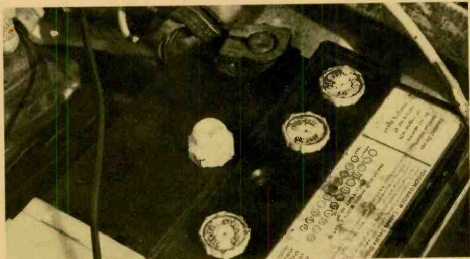
Even the best voltmeter in the world won't help you keep your car running if you don't take care of your battery. Check water level often and add only pure, distilled water.
