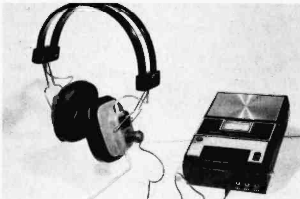
To record shortwave or other broadcasts just plug a telephone pick-up coil into a cassette recorder, then attach the pick-up to the headset.
