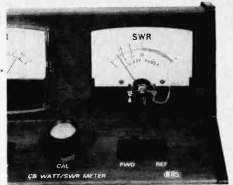
Detailed view of SWR meter face shows relation between SWR and percent of power returned. Markings show 25% of power is lost at 3:1 SWR.
