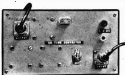
A front panel mounted crystal socket permits moderate shifting of the received frequency without internal retuning. If you use an external 6-volt supply, be sure to remove the dry cell.
