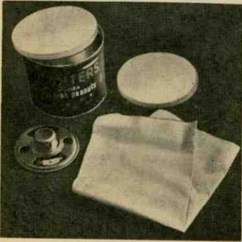
NutZee's major ingredients. Cloth covers speaker/plastic top assembly on author's NutZee; this pretties up NutZee and protects speaker cone from dust and prying fingers.
