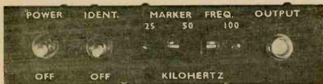
Front panel view of the Mark III details in-line arrangement for all controls. Use transfer or Datak letters for control identification to give your unit the professional appearance.
