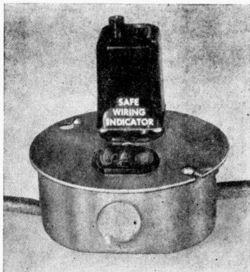
Completed indicator unit shown plugged into AC outlet. Neon bulbs are at top of case. Remember this won't work unless the ground terminal of receptacle is really grounded.
