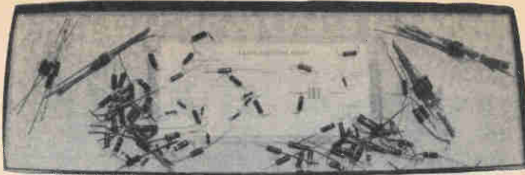
Since a great many people have trouble remembering the color code, a useful aid to sorting surplus resistors is an old tie box with the color code marked inside the lid.
