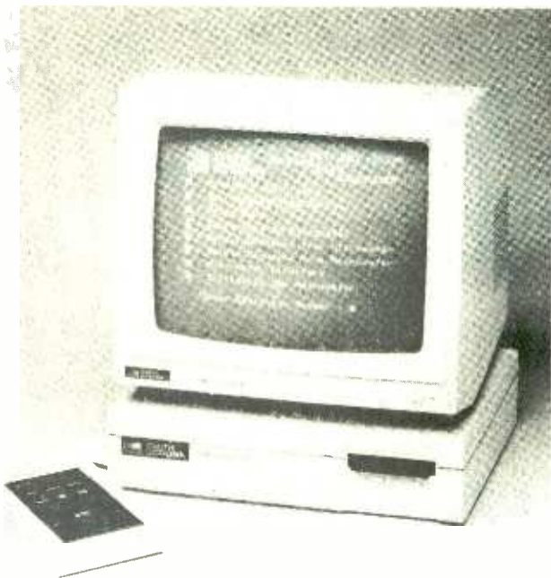
PWP Personal Word Processor by SCM lists for $500, can be used with a large number of SCM electric typewriters costing from $700 to under $300. Shown here is 12-inch monitor atop Central Processing Unit, with small Control Unit at left.
