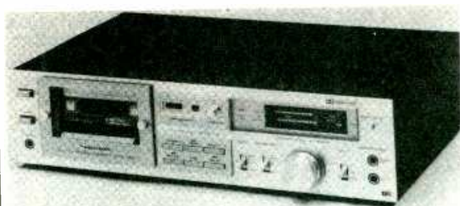
Fig 1. Here is a stereo cassette tape deck found with separate rewind, play, fast forward, record, stop and pause push buttons controlled with a solenoid circuit.
