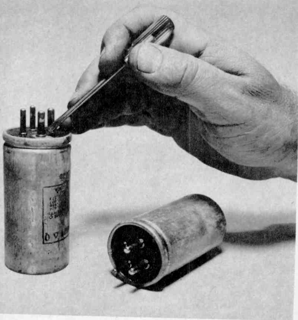
Above is shown a typical four-prong vibrator from an auto radio. It looks like a tube. These prongs should be kept clean by an occasional (bi-monthly) scraping with knife or screwdriver.
