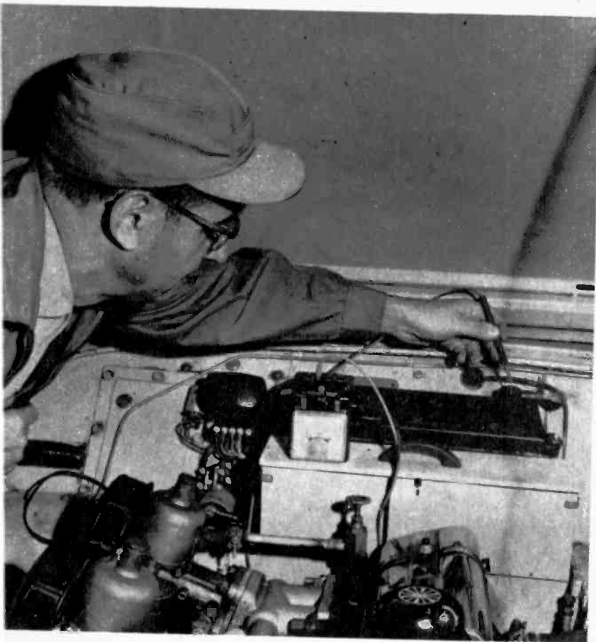
Pocket VOM is ideal for trouble-shooting in a car's electrical system. It checks voltages of battery and charging generator, wiring continuity, fuse condition, and unwanted "grounds" to vehicle's framework.
