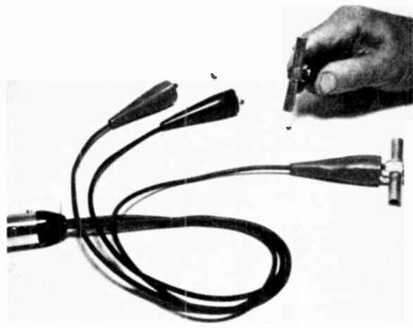
Above: These are the "probes" of the analyzer. The two insulated clips, in top left corner, go to the battery circuit. Cylindrical clips, which are split lengthwise, go to high tension leads.
