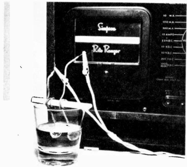
Two pennies in a very weak solution of sulphuric acid make simple primary battery. Note that the reading on the meter is only one half of a volt.
