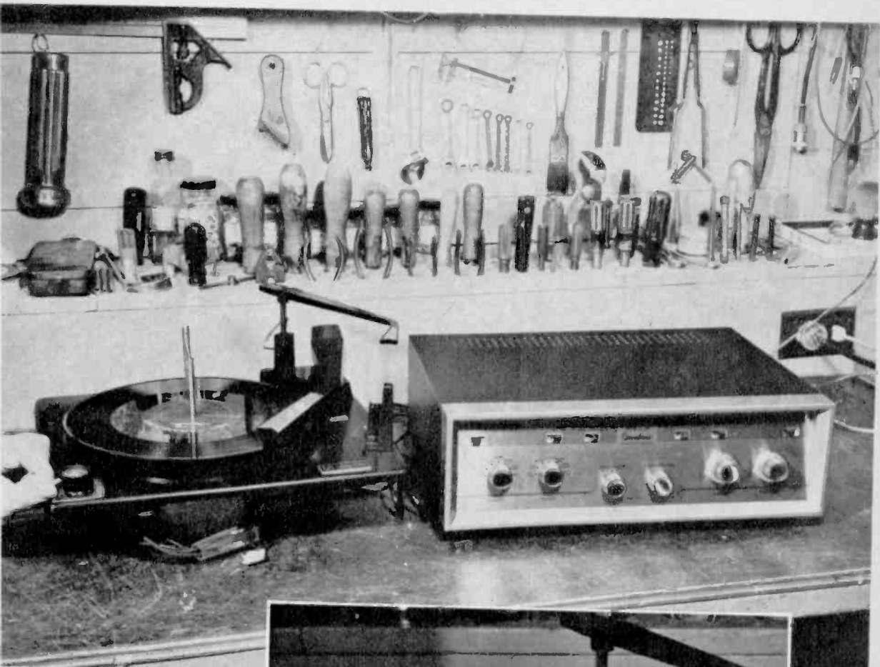
Paco SA-40 stereo amplifier is being bench tested before it is set up. Demonstration record, at left on Glasser-Steers turntable, is signal source (photo above).
