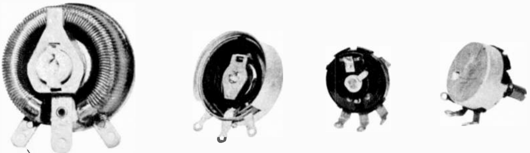
Shown in photo below, left to right: Heavy duty wire-wound potentiometer; light duty wire wound; small volume-control type pot with the cover removed; then an identical volume-control pot but with the cover.
