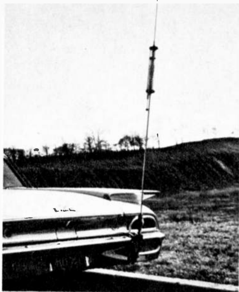
Heath RM-1 antenna, left, above, with adjustable center loading coil, enables owner of mobile equipment to work on 10, 15, 20, 40 and 80 meter bands and to take advantage of "open" conditions as they occur. Moseley MA-3 mobile whip, above right, is three-band antenna, for 10, 15 and 20 meters. The loading coils at the base and in the center are fixed. Investigate both models before you buy.
