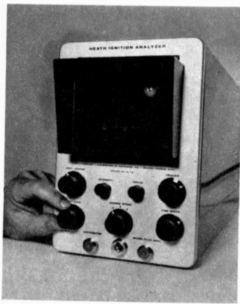
Photograph: The front panel appearance of the ignition analyzer resembles that of a standard oscilloscope. The operation of the various controls can be mastered with a little diligent practice.
