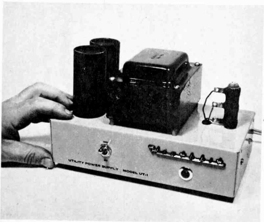
The cover is off to show power transformer (center) filter capacitors (left) and bleeder resistor (right).
