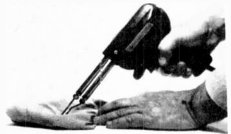
Drawing tip of iron across folded rag is an easy way of keeping the tip clean. Do with a quick, careful motion, to prevent the rag from burning.
