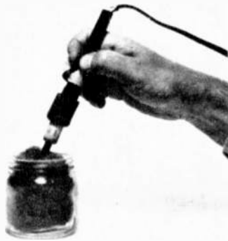
Another good cleaning agent is ball of steel wool in shallow container. Push iron (above photo) into it, twirl quickly, and tip comes out like new.
