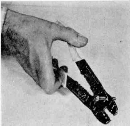
Several tapped holes in this stripper enable you to cut screws to desired length by turning screw into
