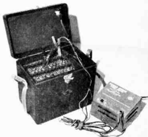
RECHARGING with 12-v. trickle charger. It takes a half hour to recharge each section.
