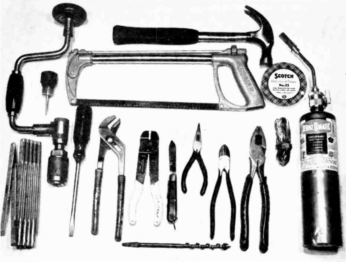
Tools used for electrical work include a folding rule, brace, screwdrivers, Channel-lock pliers, wire stripper and lug crimper, pocketknife, needle-nose pliers, linesman's pliers, propane torch, hacksaw, hammer and electrical tape.
