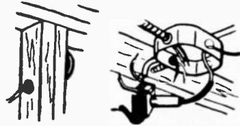
FIG. 5. Box is mounted at closet fixture and 120-v. line run to it. Two-conductor #18 is strung from door jamb to box and connected to wires from cylinder of relay.
