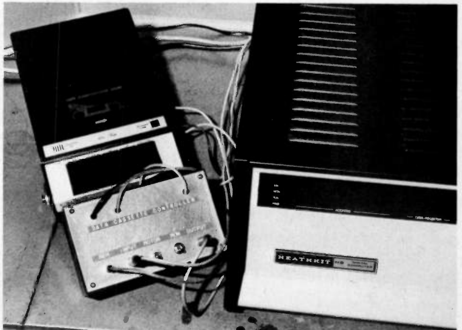
The Tape Controller connects between the computer's record interface and the cassette recorder, allowing monitoring of both the record and playback signal(s), as well as providing forward and reverse control without pulling the remote control patch cord.
