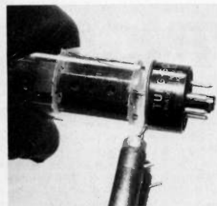
Put the loop over the part of the tube you wish to cut and hold the tube firmly. Wear gloves to keep from burning yourself on the hot glass. Next apply heat to the loop and rotate the tube until the glass cracks.
