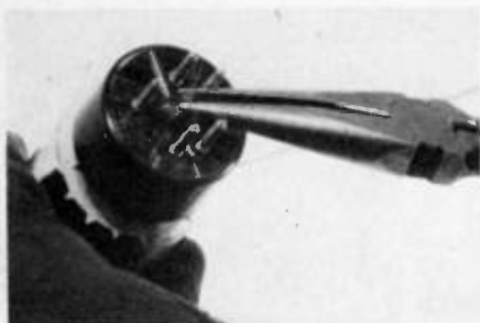
Break off the black tube-locator pin and the glass tip with some long nose pliers.
