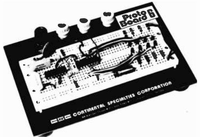
A deluxe version of the solderless breadboard, CSC's ProtoBoard has binding posts for bringing in power to the bus strips which run along the outside edges of the breadboard. The heavy base with its rubber feet can allow the builder to work virtually anywhere without creating damage to table tops and other furniture.
