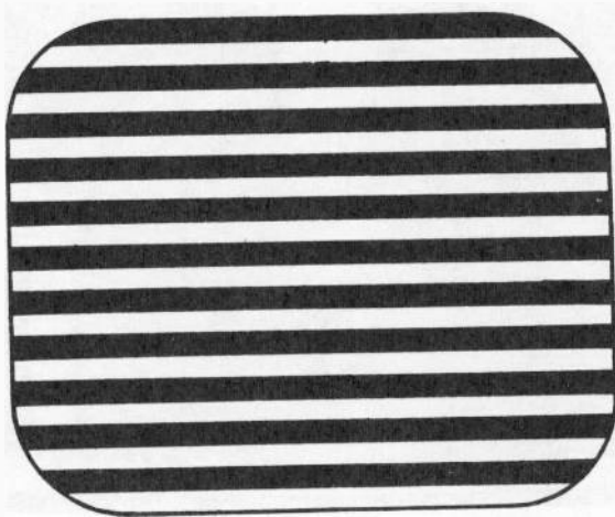
FIG. 16-27. Black and white horizontal bars for checking vertical linearity.
