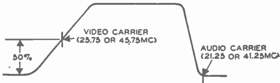
Fig. 5-7. The desired response curve of the video IF system.
