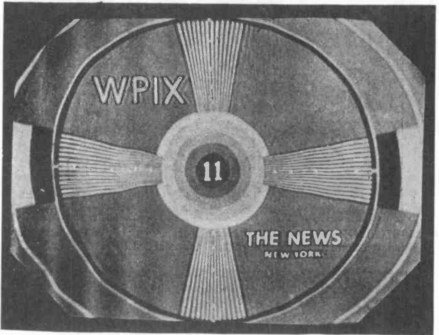
FIG. 16-18. Ripples caused by an open or wrong value of capacitor across half of the horizontal winding of the yoke.
