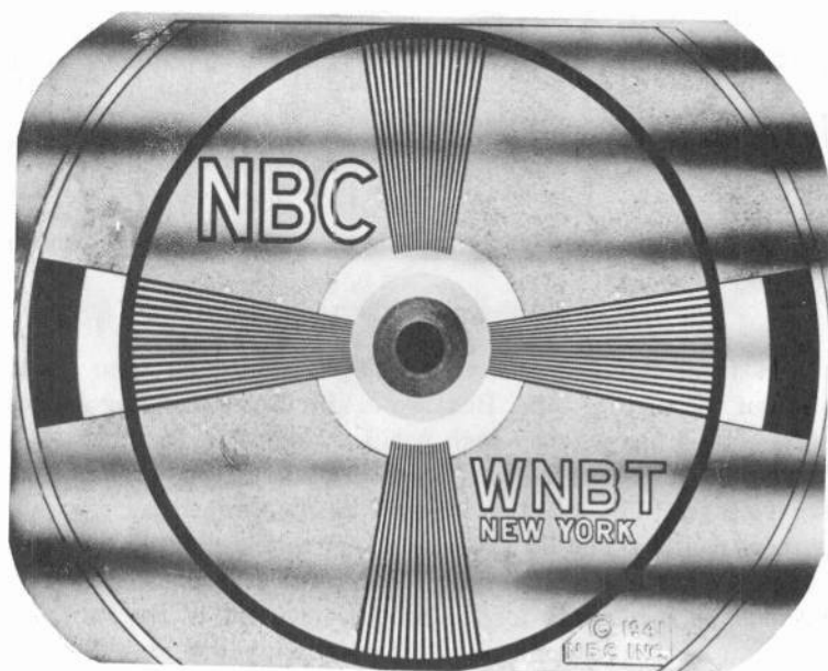
Fig. 7-33. The visual result when sound voltages reach the cathode-ray tube.
