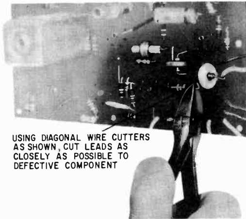
Fig. P-10. When removing parts, cut as closely to the body of the component as possible. (Courtesy Admiral Corp.)
