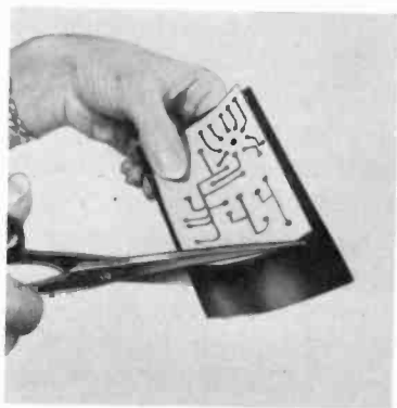
Fig. 215. The first step in the preparation of a silk-screen pattern is to cut a piece of presensitized gelatin film, slightly larger than the pattern to be reproduced.
