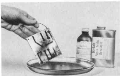
Fig. 208. Developing the exposed laminate plate.
