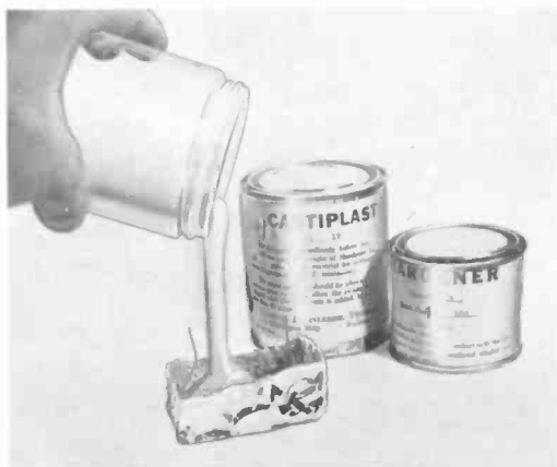
Fig. 655. The potting compound is poured around the component until it is covered.
