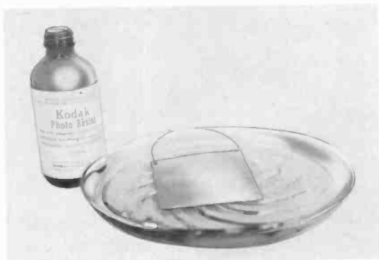
Fig. 205. (above). Dipping the laminate into photo-resist to sensitize it. (below) Removing the laminate by a wire handle attached for this purpose. (Courtesy Eastman Kodak Co.)
