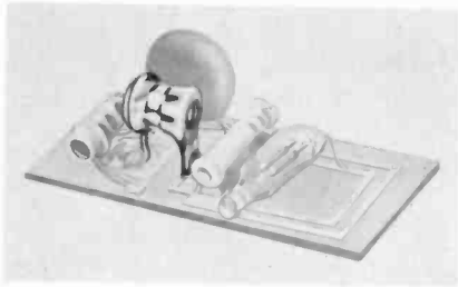
Fig. 322. A commercial printed-circuit oscillator using a piston type capacitor. (Courtesy JFD.)
