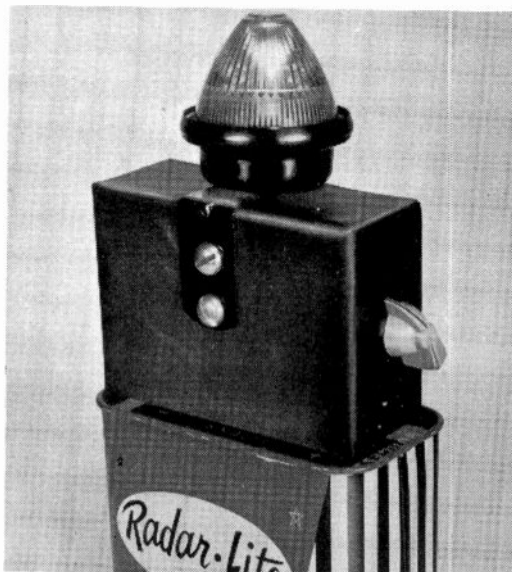
Fig. 417. The Light Flasher assembled in a small metal box and mounted on a heavy duty lantern battery.
