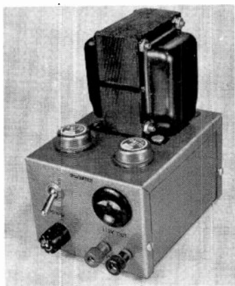
Fig. 520. Overall view of the completed Power Inverter.
