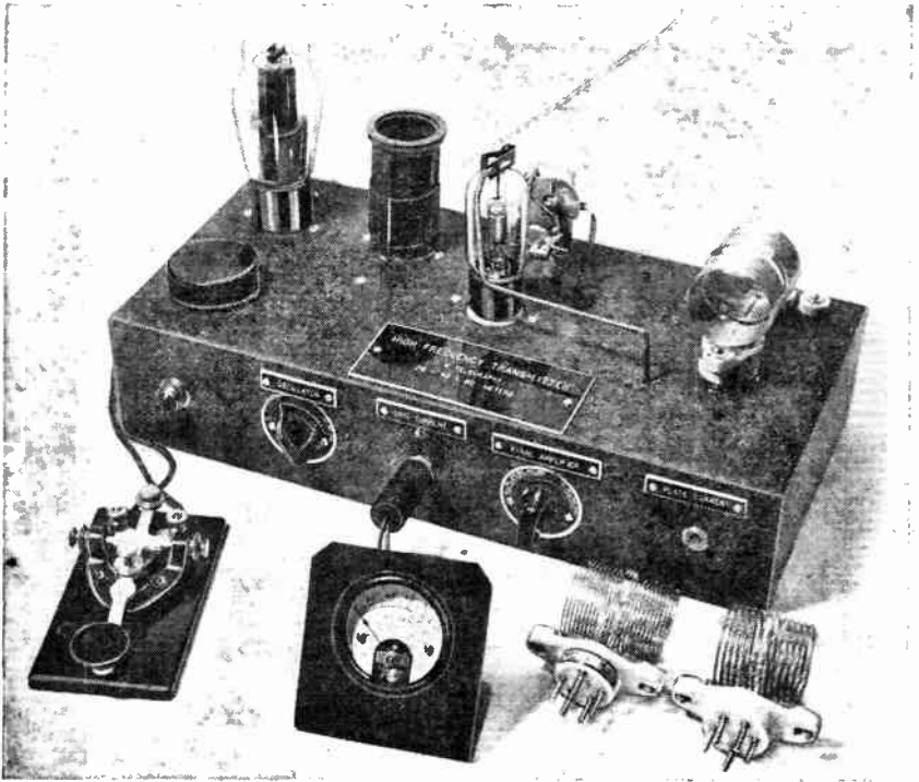
Fig. 19—Top view of the transmitter. Closed-circuit jacks permit use of one meter.
