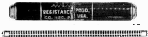
Fig. 413. Multiplier resistors used in high-voltage probes.
