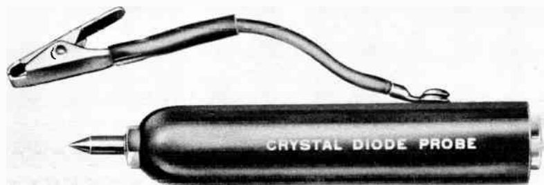
Fig. 407. Crystal-diode probe. The ground clip should be fastened as close to the test point as possible.
