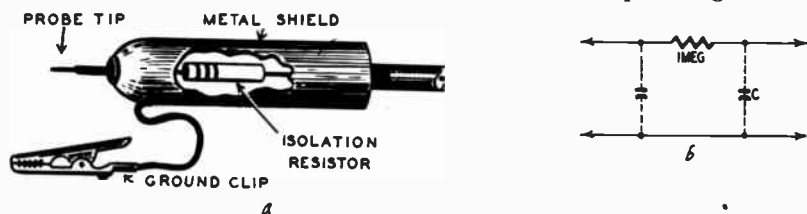
Fig. 402-a, -b. Cutaway view of isolating probe (a) and its equivalent circuit (b).
