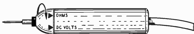
Fig. 405. Another type of combined probe. Similar to that of Fig. 404, it differs only in switch construction.
