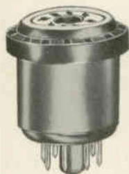
Fig. 301. Test adapter for making above-chassis voltage checks. Adapters for seven- and nine-pin miniature tubes are commercially available.
