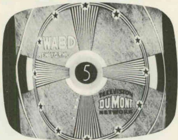
Fig. 305. Photo of test pattern indicates insufficient width.
