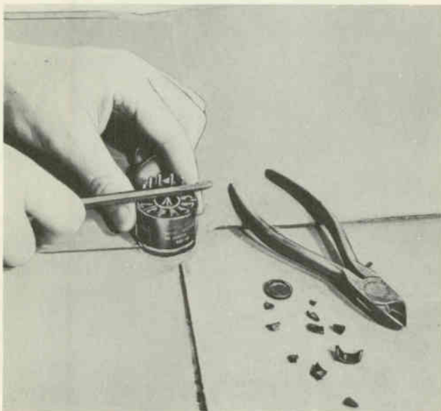
Fig. 103. Deactivating a picture tube. Drilling a hole in the keyway of the tube exposes the exhaust tip, which can then be broken.
