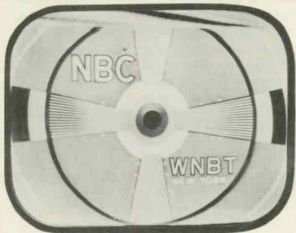
Fig. 508. Tearing out of lines at the top of the picture. The condition may be intermittent or practically continuous.
