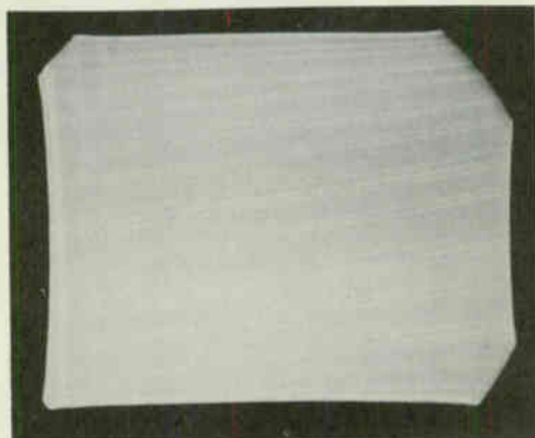
Fig. 402. How raster will look when sync pulses are not reaching the vertical oscillator. The vertical retrace lines will drift up and down, indicating that the vertical oscillator is free-running or uncontrolled.
