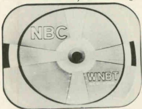
Fig. 205. Effect of horizontal nonlinearity on test pattern. Note greater width of horizontal wedge at left, compared to the corresponding wedge at the right.
