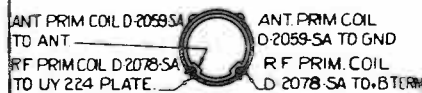
PRIMARY COIL ANT PRIM COIL - D-2059-SA (YELLOW SPOT) RF PRIM COIL - D-2078-SA (PLAIN)
