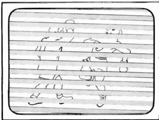
Fig. 104. This is the picture traced by the spot during the even-line field.
