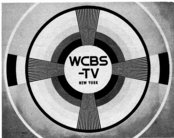
Fig. 107. Ideal test pattern. Adjust sweep size and linearity for a pattern that most closely resembles the one shown. Don't expect perfection. (CBS Television Network)
