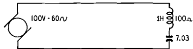
Fig. 705—The values chosen for the coil and capacitor in the circuit shown at the right are for resonance at 60 cycles.
