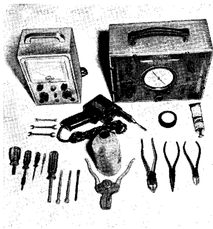
Fig. 2503—Basic equipment needed to begin a radio repair business.
