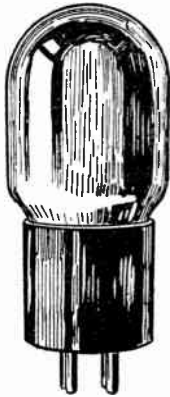
FIG. 3.—Amplifier Tube with Cylindrical Bulb.
