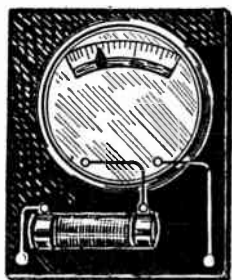
FIG. 5.—Milliammeter Used as Voltmeter.
