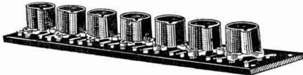
FIG. 7.—Gang Socket for Seven Tubes.
