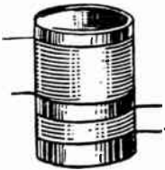
FIG. 5.—Air Core Radio Frequency Transformer.
