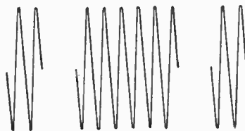
An Interrupted Continuous Wave.
