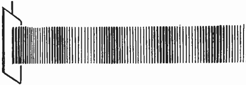
FIG. 1.—Radiation of Sound Waves from Vibrating Body.
