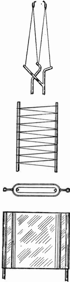
FIG. 5.—Design of a Half-Ampere Power Tube.
