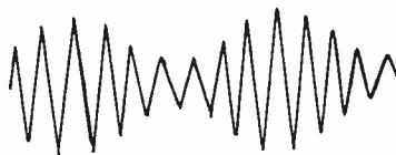
FIG. 3.—A Modulated Radio Wave.
