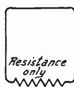
FIG. 2.—Condition of Series Resonance.
