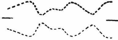
FIG. 4.—The Envelope of the Modulated Carrier.
