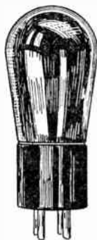
FIG. 2.—Small Half-Ampere Power Tube.
