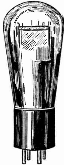
FIG. 4.—Large Type of Power Amplifier Tube.
