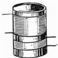
FIG. 5.—Air Core Radio Frequency Transformer.
