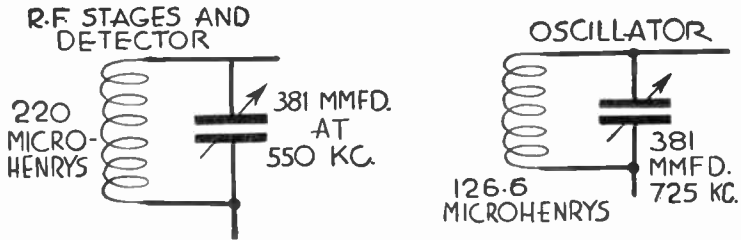
FIG. 18.—Tuning Inductances and Capacities.
