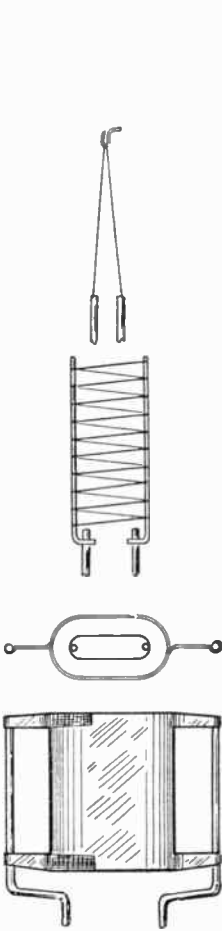
FIG. 1.—Design of an Early Type of Amplifier Tube.
