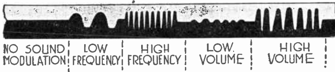
FIG. 4.—Changes in Variable Area Sound Track.
