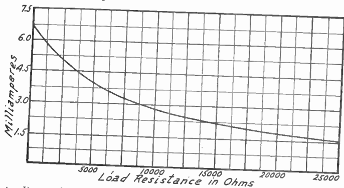
Fig. 4.—Drop of Output Current from Tube with Increase of Load When Maintaining Constant Voltage at Plate Supply Unit.
