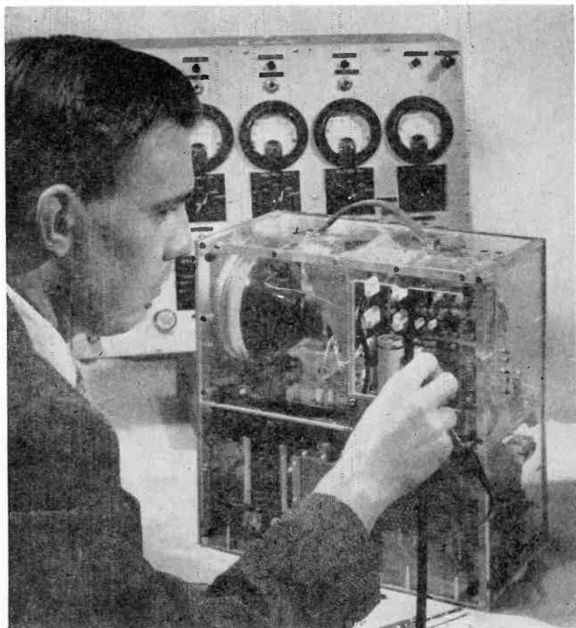
Experimental Portable TV Receiver with only one tube—the Kinescope Picture tube.
