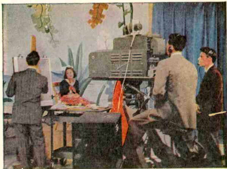
RCA color camera in operation during a color broadcast from the WNBW studios in Washington, D. C.
