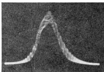
Fig. 31.—Effect of interfering station with frequency-modulated input.
