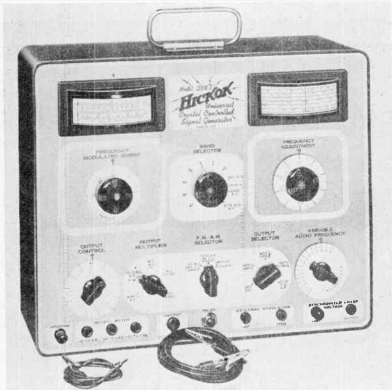
Fig. 18.—The panel of the Hickok signal generator.
