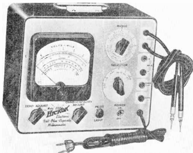
Fig. 16.—The panel arrangement of the Hickok electronic voltmeter.
