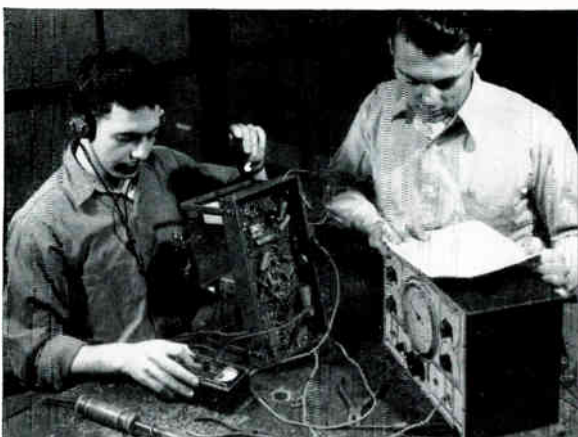
Here the students are aligning and making further tests on their Receiver. The methods taught in aligning and testing are universal and can be applied on all makes of Superheterodyne Receivers.
