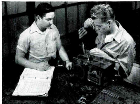
The two students pictured above are beginning to build a T.R.F. Receiver. They have checked the Circuit diagram and they are now soldering the first wire.
