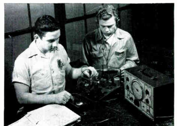
Here the finished set is being put into operation. Final adjustments are made to get the best performance from the receiver. Standard test instruments are used in making these tests and adjustments.
