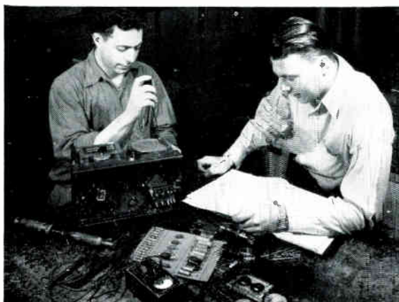
In the picture above the students are preparing the first steps in wiring up a Superheterodyne receiver. Wire, solder and parts are at hand and the next step will be soldering these parts in place.
