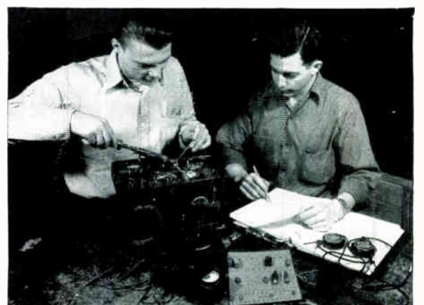
In this picture the wiring of the set is well along. Several tests have already been made as the circuit is wired one stage at a time, and it will soon be ready for final testing.
