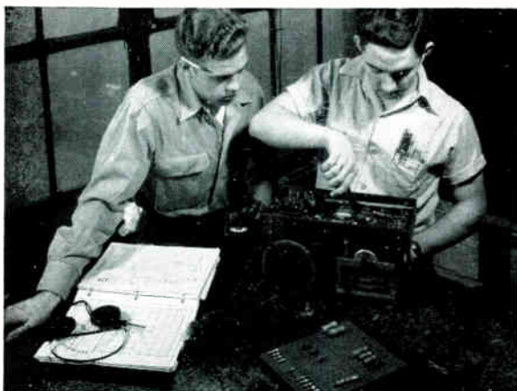
In this photo about half the wiring is complete. Notice that a large number of the parts have been removed from the board on the table and have now been soldered into their proper places.
