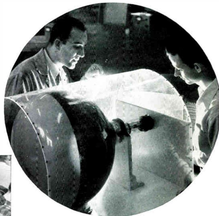
In the above photo you see an instructor giving personal instruction on the characteristics of a 20" Cathode Ray tube; one of the largest direct view Television tubes in use.
