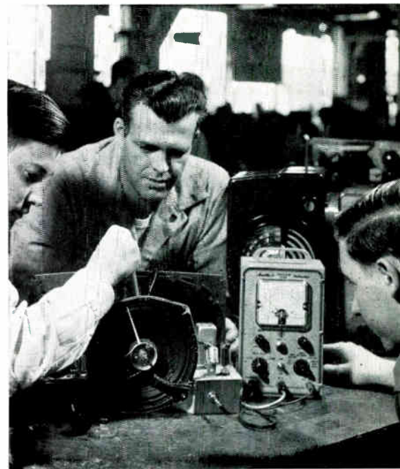
Here you see students aligning and testing an F.M. Receiving set under the supervision of an instructor. F.M. service procedure is an important part of Coyne Training.
