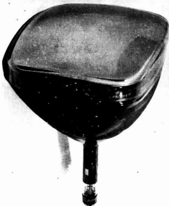
Fig. 16-2.—A television picture tube, in which are employed the principles of a triode for controlling intensity of the beam.
