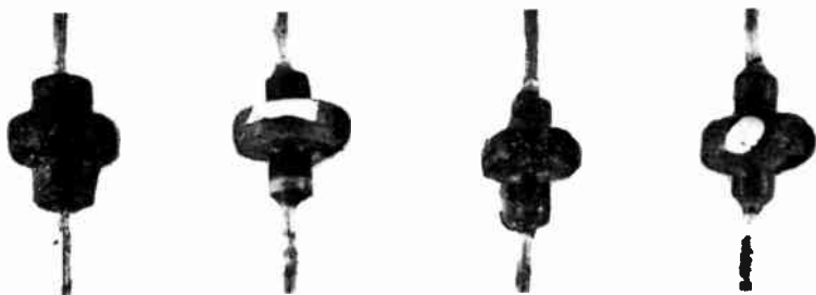
Fig. 14-2.—Peaking coils whose inductance, in combination with circuit capacitances, is resonant at a frequency around four megacycles.
