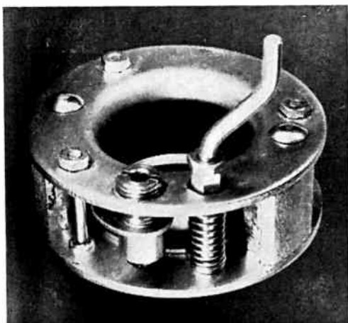
Fig. 12-1.—This permanent magnet centering and focusing device is used on television picture tubes.
