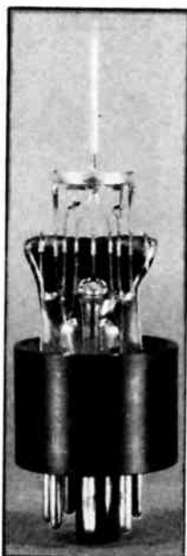
Fig. 15-10.—The coated cathode is exposed by removing the control grid.
