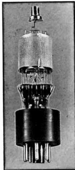
Fig. 15-4.—The pentode tube with its glass envelope removed.
