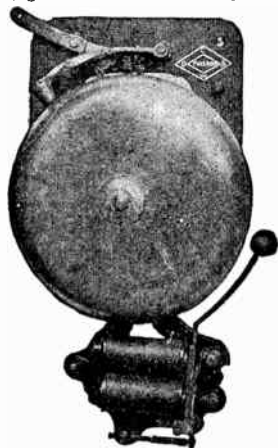
FIG. 3,208. —Partrick and Wilkins emergency gong. It operates single stroke by hand, and vibrating by battery; used by hand in emergency in giving alarms or signals. This style of bell is used for school house work.
