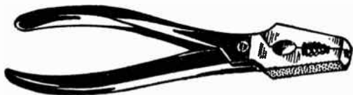
FIG. 3,404.—Carbon pliers. Carbons may be cut to any desired length by simply nicking them all around and breaking them like a glass tube. For this operation the carbon is placed in the circular opening of the pliers in such position that the nicking comes flush with the side of the pliers.
