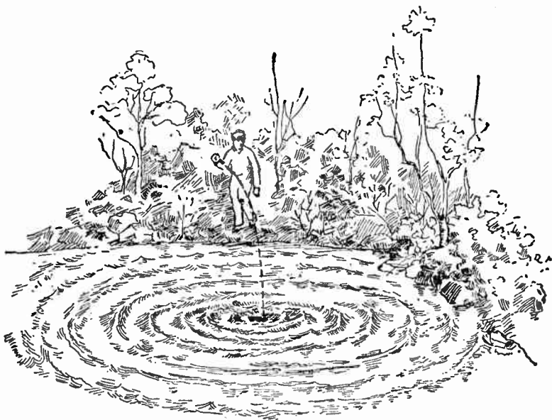
FIG. 4.—Effect of throwing a stone into still water; it produces waves which travel outwardly in expanding, concentric circles from the point where the stone enters the water or point of disturbance .
