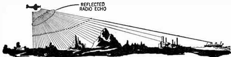
FIG. 4—An exaggerated view showing how the radio energy emitted from a radar antenna is reflected from the target. In reality only a tiny fraction of the radiated energy is reflected back to the receiver in form of an echo.
