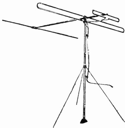
FIG. 40 —Double folded dipole antenna with reflector. An antenna of this type will give an excellent forward gain and high forward-to-back ratio. The antenna requires only one transmission line to receiver and requires no special matching network to give excellent performance on high and low bands. It is used preferably where transmitting stations are located not too far apart.
