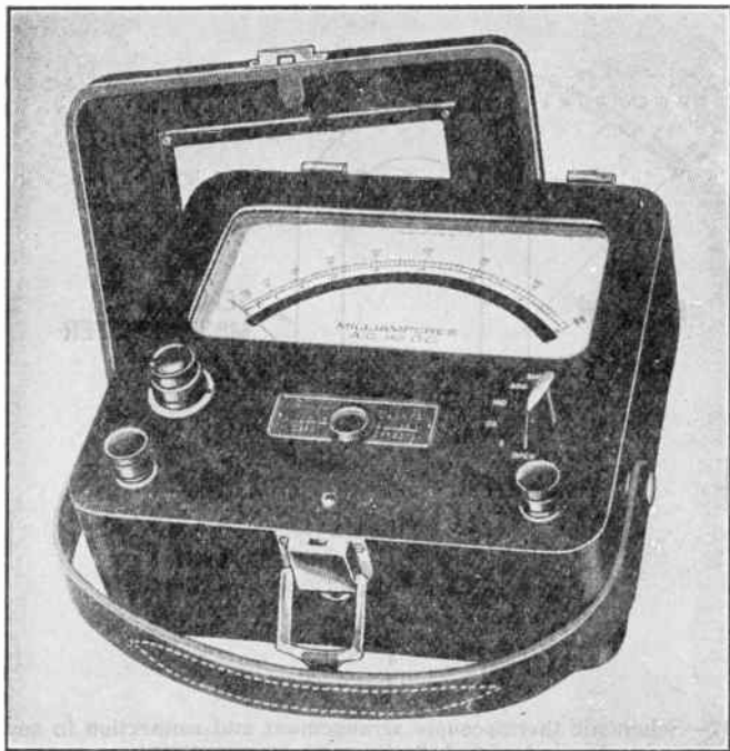
FIG. 17a —Weston Model 622 Thermo A.C.-D.C. Milliammeter.
