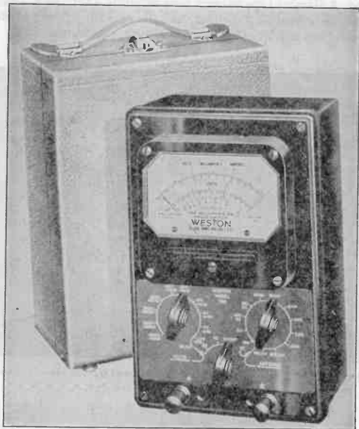
FIG. 11 —Front view of Weston Model 765 analyzer.
