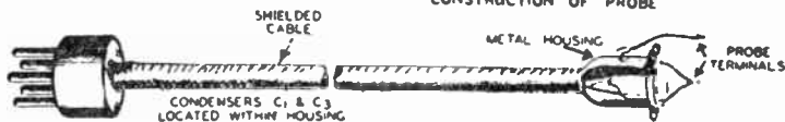
FIG. 42—Vacuum tube voltmeter arrangement in which 954 (on account of its small size) is placed at the point of measurement. In this way long leads and high input capacitances are avoided with the desirable result that measurements can be made at radio frequencies with a minimum effect on the constants of the circuit under measurement. (Courtesy Radio Corp. of America).
