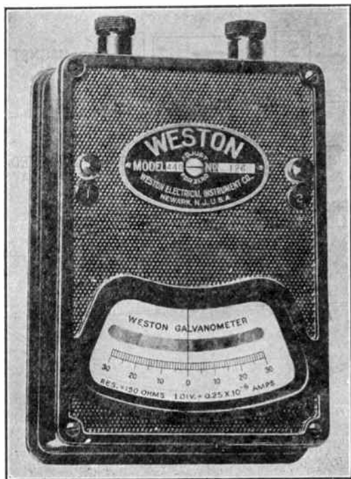
FIG. 4a —Weston model 440 movable coil galvanometer.
