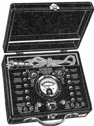
FIG. 7,404.—Supreme set analyzer. It makes available a great number of tests and provides 79 readings.
