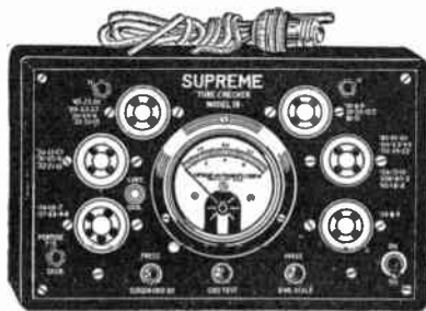
FIG. 7,400.—Supreme tube checker; portable model for either counter or portable use, with lid mounted on slip hinges, handle and detachable cord. It provides the following features: 1, tests pentode tubes and the new 2 volt 30 series tubes; 2, tests screen grid tubes with voltage closely approaching operating conditions; 3, full size 3½ in. meter, full bakelite case; 4, double scale meter, both scales calibrated; 5, large size transformer; 6, correct filament voltages applied to every type tube; 7, off and on switch.
