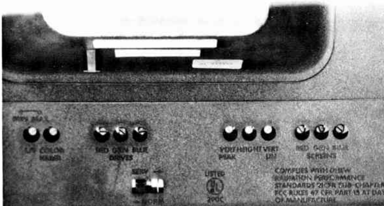
Fig. 6-4. Typical service adjustments.
