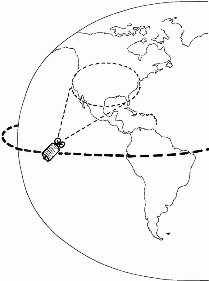
Fig. 4-8. Satellite in a geosynchronous orbit.
