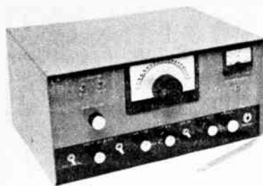
Fig. 63 — This receiver is built in a homemade aluminum cabinet. A two-tone gray and flat-black paint job has been applied. Black Dymo tape labels are used for identifying the controls in the black area, and gray labels are affixed to the gray portion of the front panel. A cut-down Jackson Brothers vernier dial mechanism (two-speed) is used for frequency readout.
