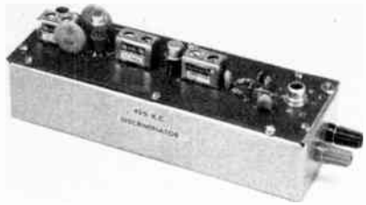
Fig. 20 — The solid-state fm adapter is constructed on a 6 × 2-inch (152 × 51-mm) etched-circuit board, mounted on a homemade chassis.
