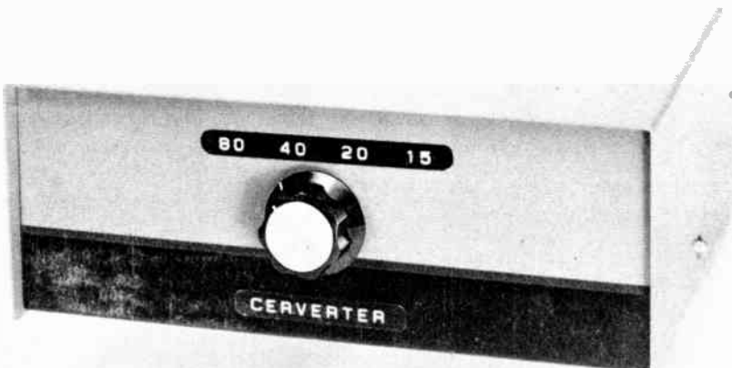
Fig. 73 — Exterior view of the high-performance converter assembly. A gray and black spray-paint finish is applied to the homemade aluminum cabinet. Lettering is by means of a Dymo tape labeler.
