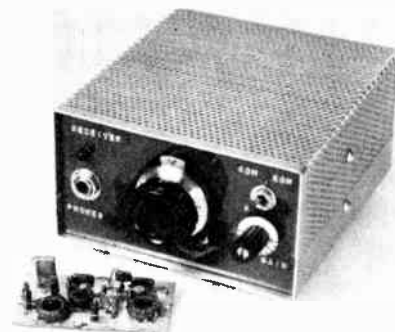
Fig. 29 — Front view of the assembled 40-meter miniature receiver. A 20-meter converter is seen in the foreground. Pc boards and parts kits for this project are available from Circuit Board Specialists, Box 969, Pueblo, CO 81002. Boards and kits for a mating transmitter (May 1978 QST, page 16) are available from the same supplier.
