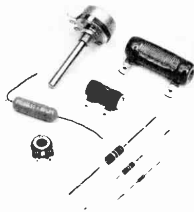
Fig. 7 — Examples of various resistors. In the foreground are 1/4-, 1/2- and 1-watt composition resistors. The three larger cylindrical components at the center are wirewound power resistors. The remaining two parts are variable resistors, pc-board mount at the lower left and panel mount at the upper center.
