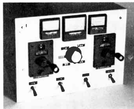
Fig. 83 — Front view of the 8877 amplifier. The non-sequential numbering of the band switch is discussed in the text. A switch is provided to allow the selection of proper bias for the mode in use at the time.
