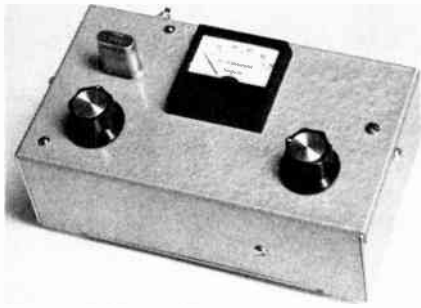
Fig. 61 — The deviation meter is constructed in a Calectro aluminum box. A four-position switch is at the lower right. The crystal plugs in on the left, with the frequency adjusting trimmer just below. A short whip or pickup wire can be plugged into the phono connector that is mounted on the back wall of the box.
