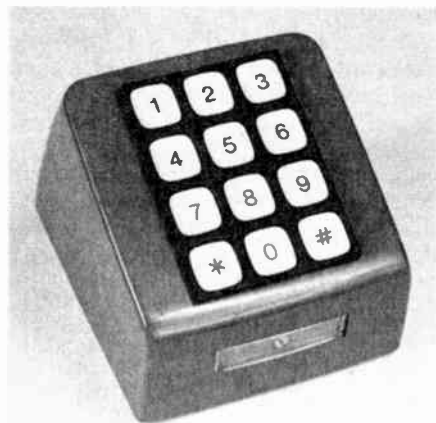
Fig. 48 — This homemade Touch-Tone generator is housed in a Western Electric sloping-front plastic box.
