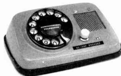
Fig. 55 — This dual-tone encoder is built in a surplus housing which was sold with the rotary dial no. TEL from John Meshna, P. O. Box 62, E. Lynn, MA 01904.
