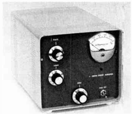
Fig. 37 — Designed and built by Dick Stevens, W1QWJ, this amplifier fills the need for a low-drive model usable with 10-watt exciters.
