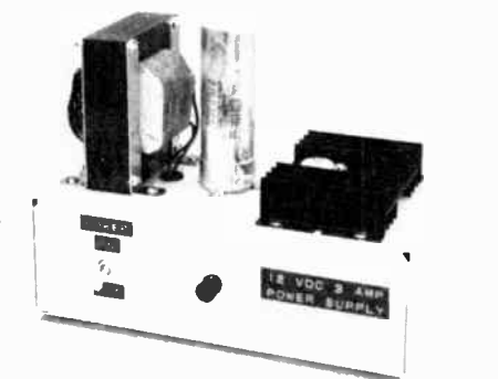
Fig. 31 — Exterior view of the 12-volt, 3-ampere, no-frills power supply.
