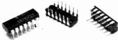
Fig. 97 — From outward appearances, these three ICs appear to be identical. Although each is a J-K flip-flop, there are differences in their characteristics. Pictured at the left is a Texas Instruments SN74H72N integrated circuit, called a J-K master slave flip-flop. Shown in the center is a Motorola MC1927P IC which is a 120 MHz ac-coupled J-K flip-flop. Both of these ICs might be considered "universal" flip-flops, for they may be used in a variety of ways. Shown at the right is a Motorola MC726P, a simple J-K flip-flop.
