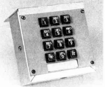
Fig. 45 — This Western Electric Touch-Tone encoder has been mounted in a 4 x 4 x 2-inch (102 x 102 x 51-mm) utility box (Bud AU-1083). Encoders are sold by most telephone supply houses, including Telephone Equipment Co., P. O. Box 596, Leesburg, FL 32748. Tel. 904-728-2730.
