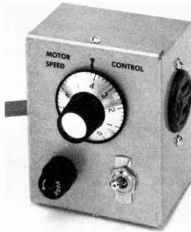
Fig. 1 — The SCR motor-speed control is housed in a small cabinet.
