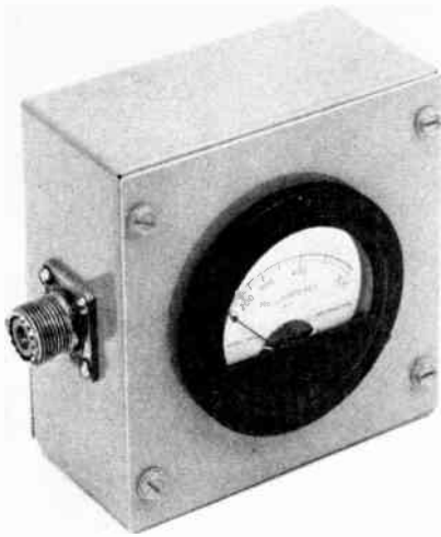
Fig. 14 — Rf ammeter mounted in a Minibox, with connectors for placing the meter in series with a coaxial line. A bakelite-case meter should be used to minimize shunt capacitance (which introduces error) although a metal-case meter can be used if mounted on bakelite sheet with a large cut-out in the case around the rim. The meter can be used for rf power measurements ( P = I^2R ) when connected between a transmitter and a nonreactive load of known resistance.
