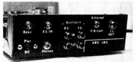
Fig. 16 — Here is a photograph of the rear panel of the processor. Layout is not particularly critical, but leads should be kept as short as possible. The use of a completely shielded enclosure is mandatory.
