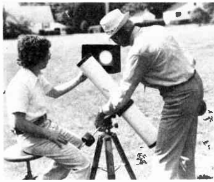
Fig. 7 — Projection viewing of the sun's image with a 4-inch (102-mm) reflector-type telescope. White-paper viewing surface is cemented in the bottom of a black-sprayed cardboard box.
