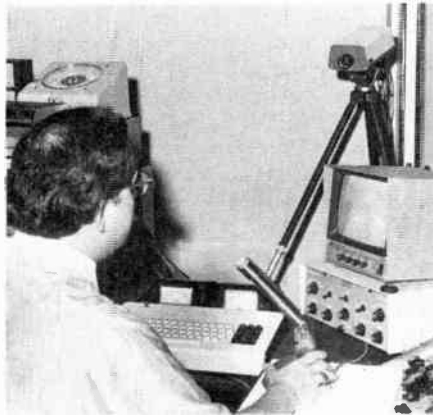
The SSTV position at W1AW as operated by ARRL Deputy Communications Manager Jim La Porta, N1CC. The operating controls are placed so that the operator has easy access to the receiver, input controls and video character generator. The lens cap is kept within reach of the camera making it easy to "cap up" at the end of a transmission to protect the vidicon. A cassette tape recorder is also kept on line to record noteworthy pictures for future use.
