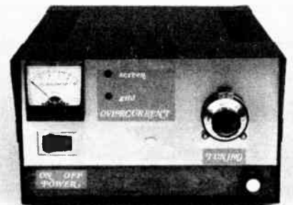
Fig. 41 — A 500-watt amplifier for the 2-meter band, complete with power supply, is housed in this cabinet. The hole plug covers a former location of a control.
