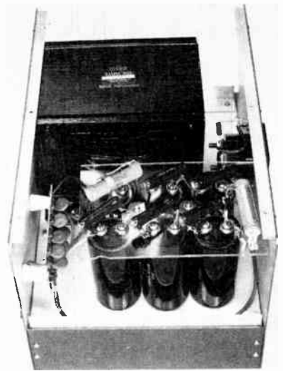
Fig. 81 — Top view of the power supply showing the technique for mounting the filter-capacitor bank. The diodes are mounted on a printed-circuit board which is fastened to the rear of the cabinet with cone insulators and suitable hardware.
