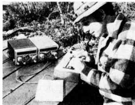
Fig. 23 — The designer, K2BLA, operating his keyboard in its intended environment. For field operation, the Gonset twins have been "solid-stated," and run 8 watts to an FET power amplifier.
