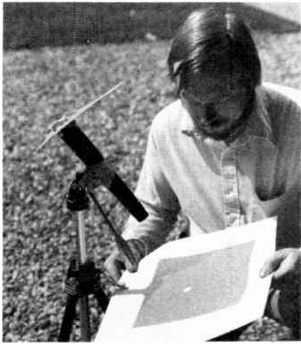
Fig. 2 — W1KXZ of the ARRL hq. staff looks for sunspots with a simple projection system. The baffle at the top end of the small telescope provides a shaded area for viewing the sun's image (light circle) on the projection surface. Sunspots large enough to affect radio propagation are easily seen with this viewing system.
