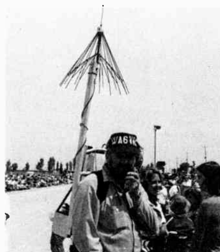
WA6VRK was one of 40 amateurs who provided communications for the five-day National Wheelchair Games in San Jose, CA. Roy used a unique rig; it consisted of two lead-acid motorcycle batteries built into a backpack. The rig was an ICOM IC-3211 into a modified discone antenna that strongly resembled a broken umbrella.
