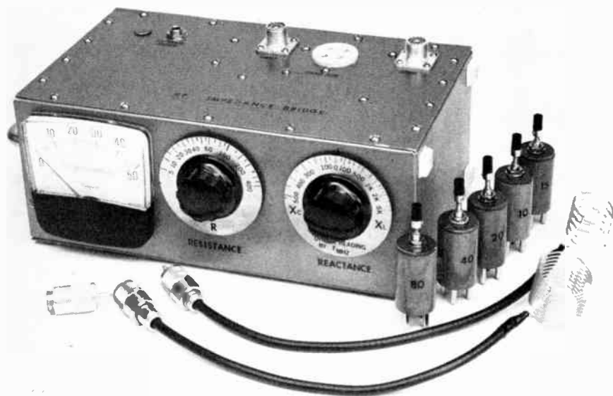
Fig. 55 — An RCL bridge for measuring unknown values of complex impedances. A plug-in coil is used for each frequency band. The bridge operates at an rf input level of about 5 volts; pickup-link assemblies for use with a grid-dip oscillator are shown. Before measurements are made, the bridge must be balanced with a nonreactive load connected at its measurement terminals. This load consists of a resistor mounted inside a coaxial plug, shown in front of the instrument at the left. The aluminum box measures 4-1/4 x 10-3/4 x 6-1/8 inches (108 x 273 x 156 mm) and is fitted with a carrying handle on the left end and self-sticking rubber feet on the right end and bottom. Dials are Millen no. 10009 with skirts reversed and calibrations added.
