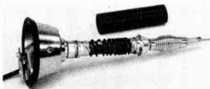
Fig. 22 — The new coil is tapped two turns from the base end. It may be necessary to file the coil ends so that the assembly will fit in the phenolic covering.
