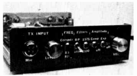
Fig. 14 — Front-panel view of a prototype compandor system. As outlined in the text, considerable flexibility has been designed into the system. Various modes of operation can be selected at a flip of the switch.
