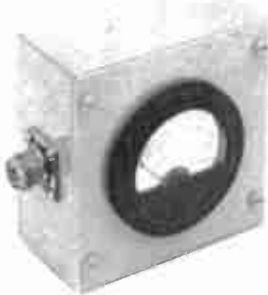
Fig. 17-10 — Rf ammeter mounted in a Minibox, with connectors for placing the meter in series with a coaxial line. A bakelite-case meter should be used to minimize shunt capacitance (which introduces error) although a metal-case meter can be used if mounted on bakelite sheet with a large cut-out in the case around the rim. The meter can be used for rf power measurements ( P = I^2R ) when connected between a transmitter and a nonreactive load of known resistance.
