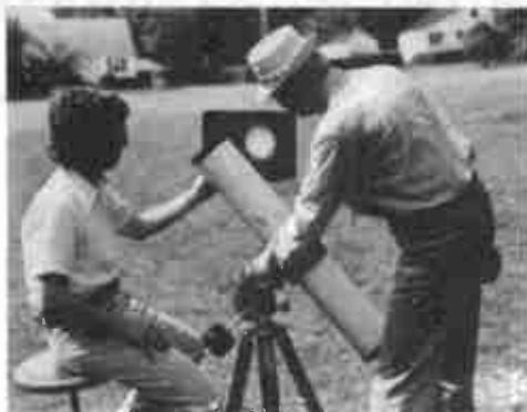
Projection viewing of the sun's image with a 5-inch reflector-type telescope. White-paper viewing surface is cemented in the bottom of a black-sprayed cardboard box.
