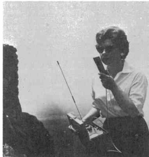
Fig. 10-1 – Effective portable operation can be realized when using lofty locations for vhf or uhf. Here, W1CKK is shown operating a battery-powered, 150-mW output, 2-meter transceiver. With only a quarter wavelength antenna it is possible to communicate with stations 25 miles or more away. Low-power transistor equipment like this unit will operate many hours from a dry-cell battery pack.
