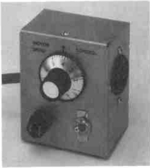
Fig. 1 — The SCR motor-speed control is housed in a small cabinet.
