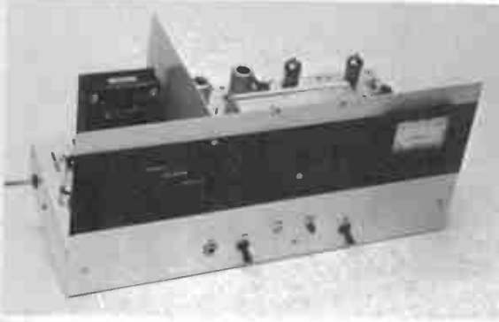
Fig. 7-7 — Panel view of the 2-meter transverter. This version is patterned after a transmitting converter design by K9UIF. The on-off switches for ac and dc sections of the power supply are mounted on the front panel of the unit as are the pilot lamps and plate meter for the PA stage. The tuning controls for the various stages are accessible from the top of the chassis.
