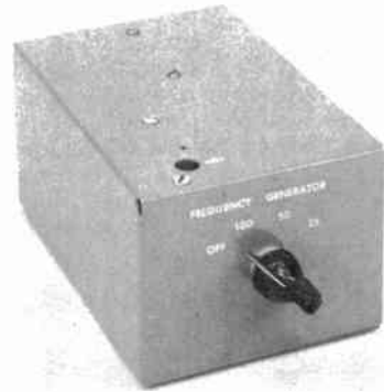
Fig. 17-29 — Frequency marker generating 100-, 50-, or 25-kHz intervals. Battery power supply (two "D" cells) is inside the cabinet, a 3 X 4 X 6-inch aluminum chassis with bottom plate. The trimmer capacitor for fine adjustment of frequency is available through the hole in the top near the left front.
