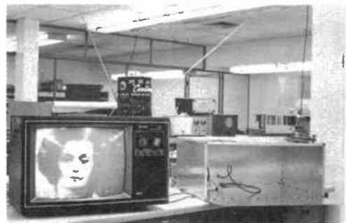
Lab simulation of TVI tests discussed in the text. A dummy load placed next to the "rabbit ears" served as the transmitting antenna.
