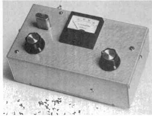
Fig. 17-56 — The deviation meter is constructed in a Callectro aluminum box. A four-position switch is at the lower right. The crystal plugs in on the left, with the frequency adjusting trimmer just below. A short whip or pickup wire can be plugged into the phono connector that is mounted on the back wall of the box.
