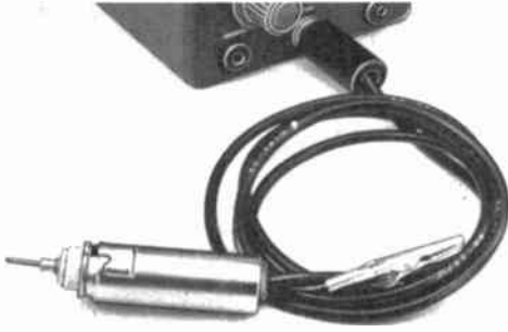
Fig. 17-52 — Rf probe for use with an electronic voltmeter. The case of the probe is constructed from a 7-pin ceramic tube socket and a 2 1/4-inch tube shield. A half-inch grommet at the top of the tube shield prevents the output lead from chafing. A flexible copper-braid grounding lead and alligator clip provide a low-inductance return path from the test circuit.
