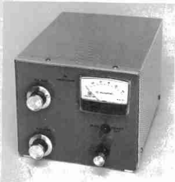
Fig. 7-3 — The 6-meter transverter, with shield cover in place. Large knobs are for amplifier tuning and loading. Small knob, lower right is for a meter sensitivity control. The meter switch is just above it.
