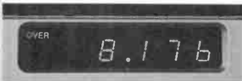
Fig. 6-12 — A 5-digit readout using light-emitting diodes.
