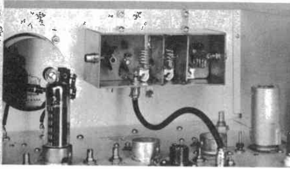
Fig. 7-9 — Inside view of the converter. Shields are used between the rf amplifier input and output circuits, and between the latter and the mixer input circuit. The cable entering the bottom side of the enclosure carries the oscillator injection energy. Output to the associated receiver or transceiver is taken through the jack to the left.
