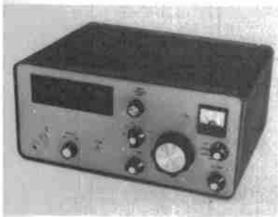
Front view of the communications receiver built by WA1JZC. The receiver controls are grouped at the right side of the front panel, with the digital readout occupying the left side.
