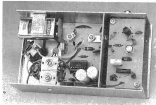
Fig. 17-58 — The dual op amp is located just below the center. Meter terminals are used as a convenient support for the amplifier pc board. The oscillator board is at the right, held in place by means of metal spacers.
