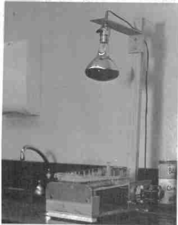
Fig. 18-10 — A homemade stand for processing etched-circuit boards. The heat lamp maintains the etchant-bath temperature between 90 and 115 degrees, F. and is mounted on an adjustable arm. The tray for the bath is raised and lowered at one end by the action of a motor-driven eccentric disk, providing the necessary agitation of the chemical solution. A darkroom thermometer monitors the temperature of the bath.
