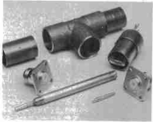
Fig. 22-24 — Major components of the line sampler. The brass T and two end sections are at the back of the picture. A completed probe assembly is at the right. The N connectors have their center pins removed. The pins are shown with one inserted in the left end of the inner conductor and the other lying in the right foreground.
