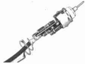
Fig. 17-54 — Inside the probe. The 1N34A diode, calibrating resistor, and input capacitor are mounted tight to the terminal strip with shortest leads possible. Spaghetti tubing is placed on the diode leads to prevent accidental short circuits. The tube-shield spring and flexible-copper grounding lead are soldered to the cable braid (the cable is RG-58/U coax). The tip can be either a phone tip or a short pointed piece of heavy wire.
