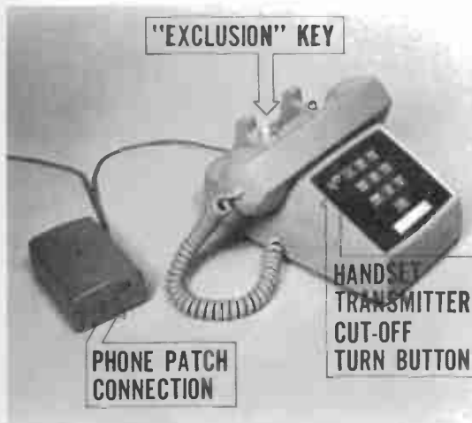
Fig. 15F-1 — The voice coupler, to the left of the touch-tone telephone, is supplied by the telephone company. The coupler is normally fixed to a wall or desk, and contains a jack for connection of the amateur's phone patch.
