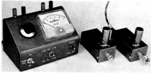
Fig. 21-27—Two diode noise generators and (left) their power supply. Useful generator range is (right) 7 to 90 Mc. and (center) 90 to 450 Mc.
