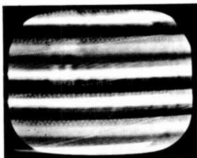
Fig. 23-6—"Sound bars" or "modulation bars" accompanying amplitude modulation of an interfering signal. In this case the interfering carrier is strong enough to destroy the picture, but in mild cases the picture is visible through the horizontal bars. Sound bars may accompany modulation even though the unmodulated carrier gives no visible cross-hatching.
