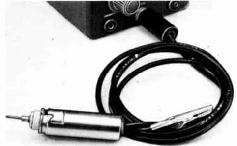
Fig. 21-35—The r.f. probe is used in conjunction with a vacuum-tube voltmeter. The case of the probe is constructed from a 7-pin ceramic tube socket and a 2¼-inch tube shield. A half-inch grommet at the top of the tube shield prevents the output lead of the probe from chafing. The flexible copper-braid grounding lead and alligator clip provide a low-inductance return path from the test circuit. The d.c. output of the probe goes to the phone plug, which plugs into the d.c. input jack of the v.t.v.m.
