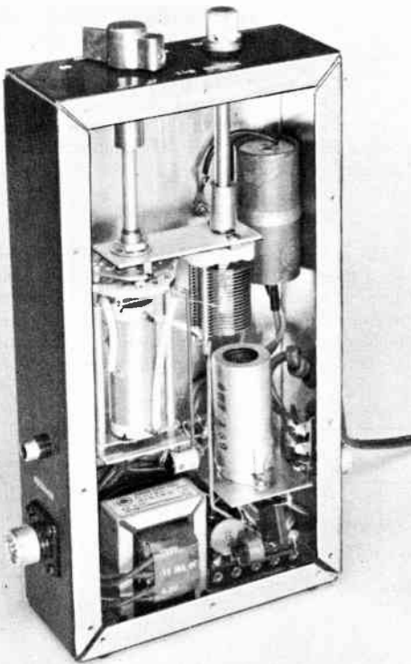
Fig. 22-3—The electronic t.r. switch is built in a 5 \times 9 \times 2\frac{1}{2} -inch chassis. Although two receiver outlets are shown on the near face (a phono jack and a coaxial receptacle), only one is required, depending upon one's choice of cable termination.
