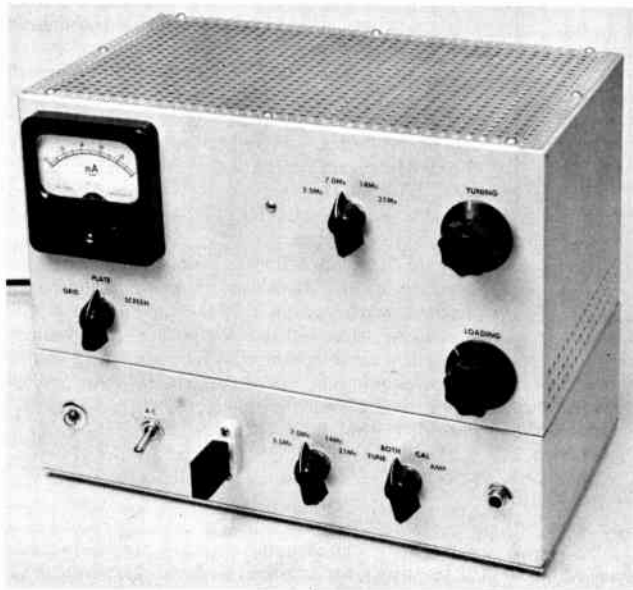
Fig. 6-35—The four-band 50-watt transmitter is a two-tube unit much superior to the "simple 1-tube" transmitters often recommended for newcomers to amateur radio. The cabinet combines a chassis and an aluminum "utility box."
