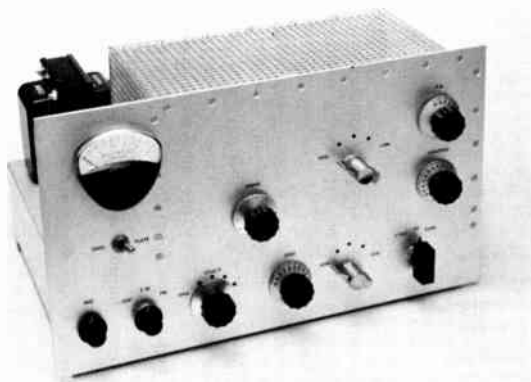
Fig. 6-48—This 75-watt transmitter can be increased to 120 watts by changing voltage-regulator tubes in the power supply; an audio section is included for screen-grid modulation of the amplifier.
