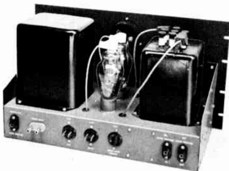
Fig. 8-21—A typical Class B modulator arrangement. This unit uses a pair of 811As, capable of an audio power output of 340 watts, and includes a splatter filter. The modulation transformer is at the left and the splatter choke at the right. All high-voltage terminals are covered so they cannot be touched accidentally.
