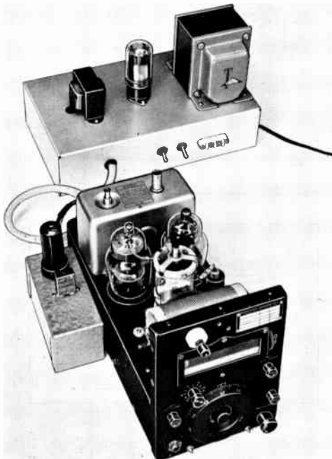
Fig. 6-91—The complete Novice setup, in this case using the 80-meter (BC-696) transmitter. Note the key jock at the lower-left corner of the transmitter panel. The crystal oscillator is connected to the transmitter oscillator-tube socket with a short length of cable terminating in an octal plug. A small notch should be cut in the transmitter cover to provide clearance for the cable when the cover is installed.
