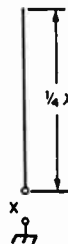
Fig. 19-29—The quarterwave whip at resonance will show a pure resistance at the feed point X.
