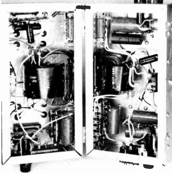
Fig. 19-49—Only electrical connections between the two chassis are through fastenings and the +12-volt lead (top center). Construction of the units is simplified by generous use of sub-assemblies (outlined in dot-and-dash lines in Fig. 19-50). The sub-assemblies are made up on multiple tie-point strips, wired and put in place. Bridge rectifier section, CR 3 through CR 14 , is made on four tie-point strips arranged in a square (lower left). The insulated terminal on the low-voltage supply (upper right) receives the +12 volts from the battery.
