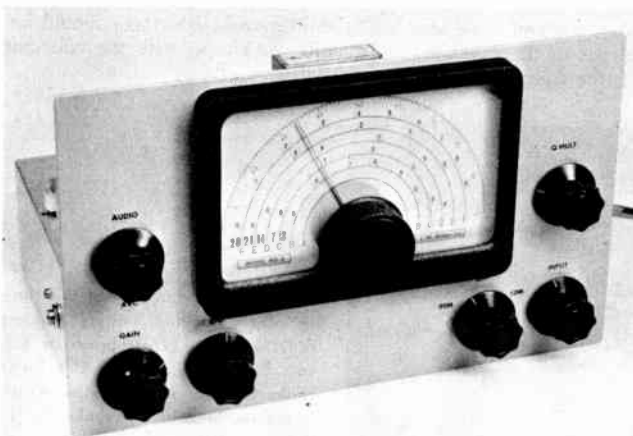
Fig. 5-38—This five-tube receiver is band switched, 3.5 through 30 Mc. The oscillator tuning dial (Miller MD-8) has a two-speed drive. Input stage is a 7360 mixer with r.f. Q multiplication.
