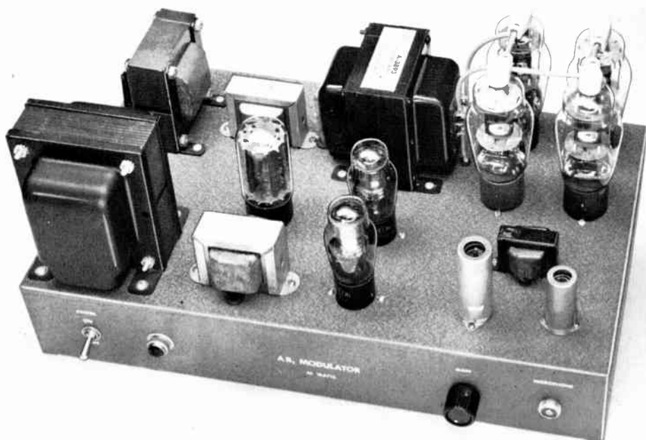
Fig. 8-15—A 50-watt modulator, using four 1625-type tubes in Class AB 1 . With higher plate voltage and a larger modulation transformer, the tubes can deliver up to 140 watts of audio power.
