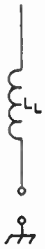
Fig. 19-34—Placing the loading coil at the center of the whip antenna, instead of at the base, increases the radiation resistance, although a larger coil must be used.
