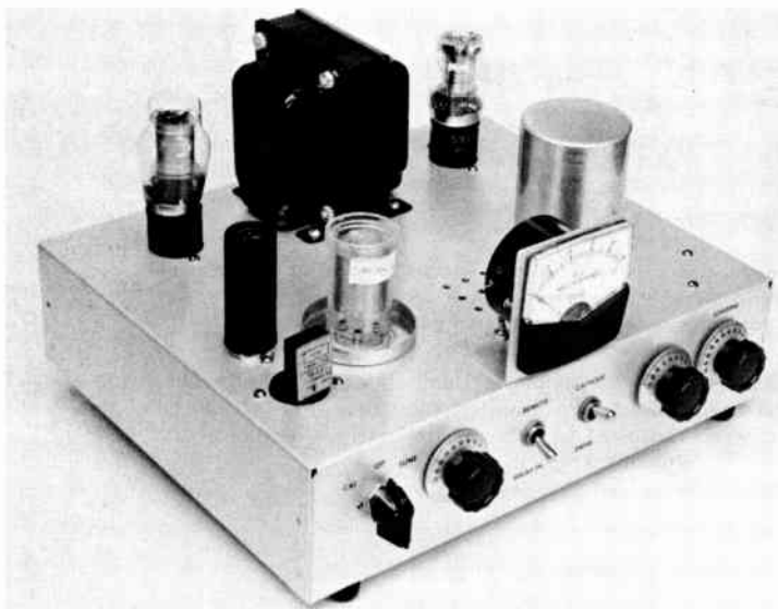
Fig. 6-40—The inexpensive 75-watt transmitter is a two-tube five-band crystal-controlled transmitter; v.f.o. control can be added at any time. To simplify construction and testing, plug-in coils are used, housed in the two shield cans (Millen 80011 or Miller S-42 with S-42C base). The crystal-oscillator tube, a 12BY7, is housed in the black tube shield at the left; the 1625 amplifier tube is mounted under the chassis.
