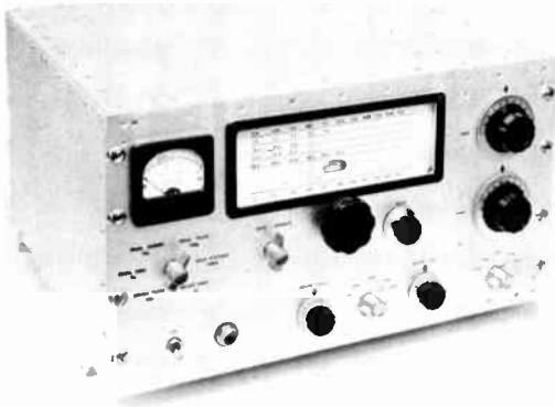
Fig. 6-60—The 450-watt c.w. transmitter is mounted on I beams of Reynolds T-shaped aluminum to allow air to be drawn in at the bottom and cool the 4E27A/5-125B final by convection. Controls along the bottom, from left to right, are the power switch and associated pilot light, driver plate tuning, exciter band switch, exciter tuning and final band switch. Above, from left to right, are the meter switch, spot-operate control, v.f.o. tuning, final drive control and final loading. Final plate tuning control is at the upper right. The v.f.o. dial is an Eddystone 898, the pointer knobs are National, and all other dials are Johnson. (Built by Walter Lange, W1YDS, West Hartford, Conn.)
