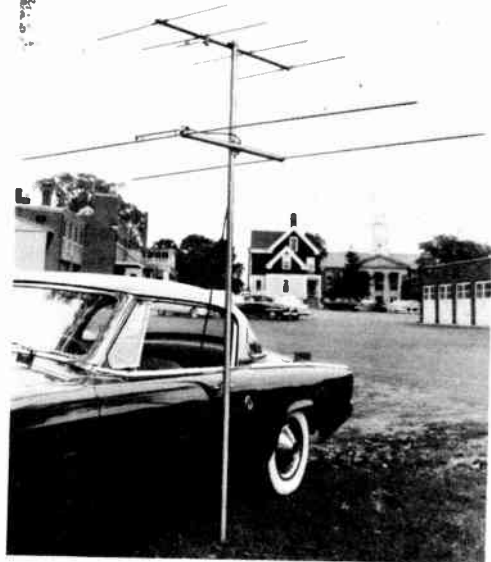
Fig. 18-5—Two-element 50-Mc. and four-element 144-Mc. arrays designed for portable use. Support is sectional TV masting clamped to car door handle. Elements of 50-Mc. array are made in three sections, for stowing in back of car. Antenna for 144 Mc. is cut-down TV array. Both use gamma match, as shown in Fig. 18-6.
