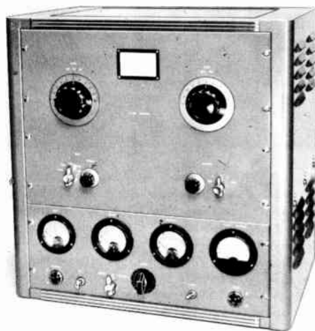
Fig. 6-72—The kilowatt 4-400A amplifier and its control unit are mounted in a 21-inch gray hammer-tone rack cabinet (Bud CR-1727). Shelf brackets (Bud SA-1350) are mounted on both sides of the cabinet to hold the amplifier chassis. Below the meters, from left to right: filament pilot light, key-type a.c. switch, Class AB/C bias switch, screen autotransformer, plate switch and plate pilot light.
