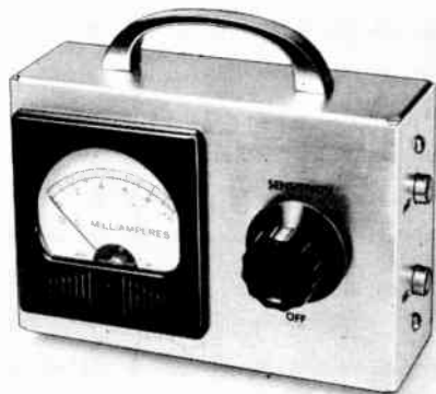
Fig. 19-41—A front view of the field-strength meter. Sensitivity control R_1 is to the right of the 0-1 indicating meter. Antenna input and output connectors are mounted on the right end of the box.
