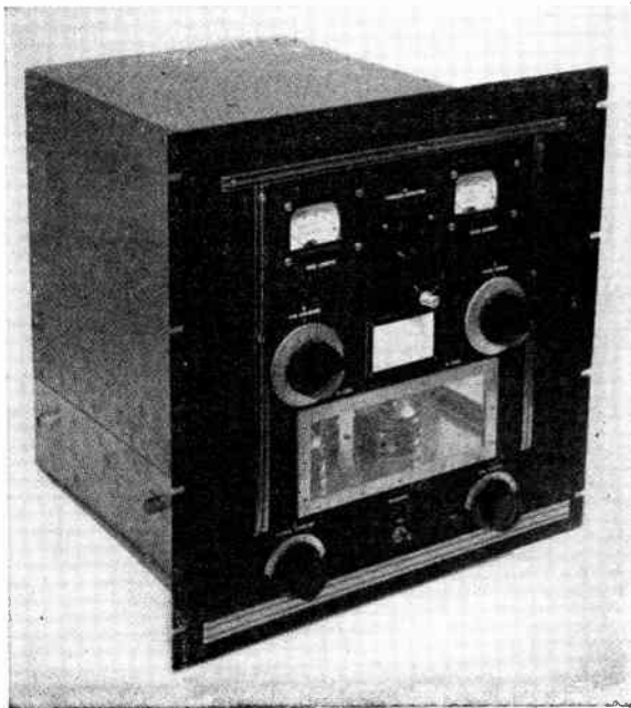
Fig. 6-87 — Front view showing the panel layout. Controls along the bottom are S_2 (coarse coupling), filament switch and grid-tuning. Above the window are the controls for C_{13} (fine coupling) and plate tuning. Between the meters is the counter dial on L_4 . The input and output connectors are along the left drop of the chassis. The hole in the center of the perforated top cover is for access to F_n . The chrome strips cover the 6-32 machine screws that fasten the angle to the panel. National CFA chart frames are used to cover the meter openings, and one is placed between the plate and output controls to use as a tuning chart. The bottom of RFC_2 shows between the tube bases, through the screened opening.
