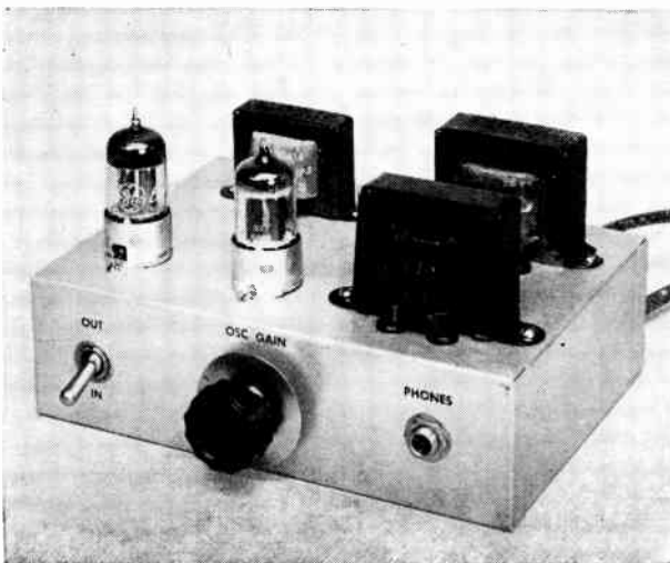
Fig. 8-12 — A combination c.w. monitor and code-practice oscillator that can be used without modification of the receiver or transmitter.
