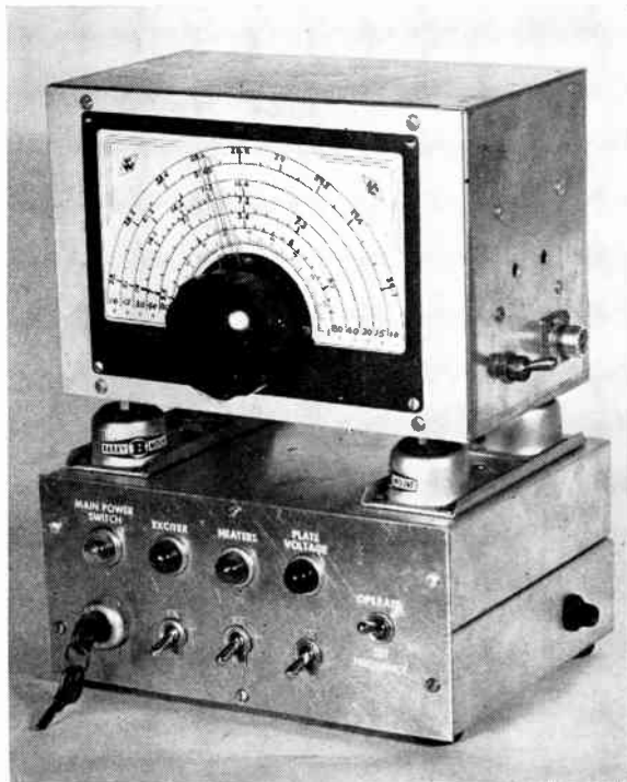
Fig. 6-73—The VFO remote tuning unit and control box. The tuning unit is enclosed in a 5×6×9-inch aluminum box mounted on shock absorbers. The control-unit enclosure is made up of two 7×9×2-inch aluminum chassis, bottom to bottom. The range-control switch and remote cable connector are mounted on one end of the tuning unit. A fuse holder projects from the end of the control unit.
