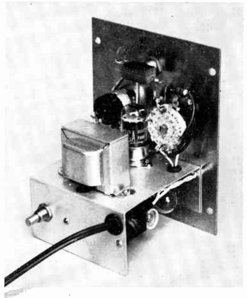
Fig. 21-27 — Inside view of the audio oscillator. The a.c. switch, S 3 , is mounted on the output control at the left. The ceramic capacitors in the frequency-determining circuits are mounted on the rotary switch, S 1 , at the right. S 2 is above the tube, and T 1 is on the near edge of the chassis, which is a U-shaped piece of aluminum 3½ inches deep with 1½ inch lips. R 1 is mounted on the near lip at the left.
