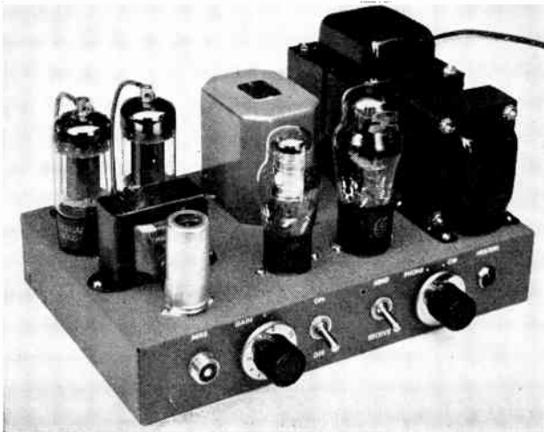
Fig. 9-13 — A modulator for transmitters operating at plate input up to 50 watts. The speech amplifier and modulator are at the left in this view; power supply components are at the right.
