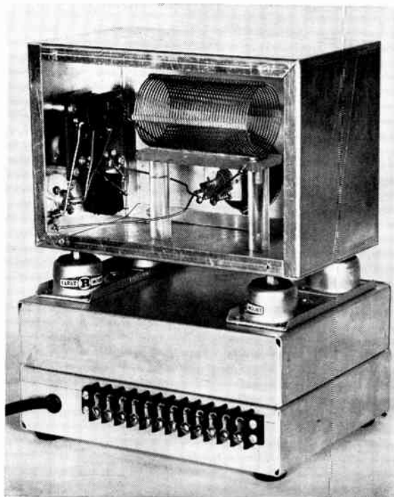
Fig. 6-74 — Rear view of the tuning unit showing the mounting of the inductor on polystyrene sheet and rods and the arrangement of other components. Ceramic trimmers, mounted on the insulating panel at the left, were later replaced with air trimmers ( C_2 and C_3 ).
