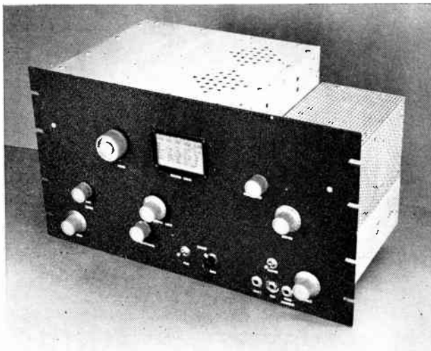
Fig. 17-5—The high-powered 2-meter rig, with shielding enclosures in place. The small unit at the right houses the tripler and driver stages.
