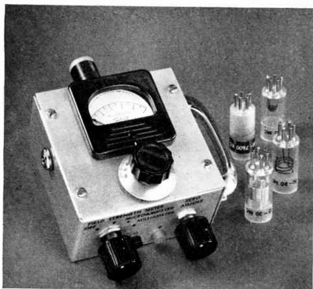
◆ Fig. 21-33 — Transistorized field-strength meter and monitor. Plug-in coils cover the amateur bands from 1.8 to 50 Mc. The function switch, meter pin jacks, and zero-adjust control are on the near edge of the 2 × 4 × 4 inch aluminum box. The headphone jack, on the left side, is insulated from the box. The dial on top is the tuning control. ◆
