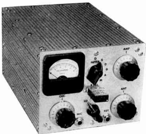
Fig. 19-17 — Front view of the 6-band mobile transmitter. The control knob for S_2 is located in between the meter and the dial for C_3 and C_4 . S_1 is directly below the crystal socket, with the knobs for C_2 and C_5 to the left and right, respectively. J_1 and J_5 are at the bottom of the 4\frac{7}{8} \times 6\frac{1}{4} -inch panel. The perforated aluminum cover is 9\frac{1}{16} inches deep and has a hole punched in the left side to permit adjustment of C_1 .
