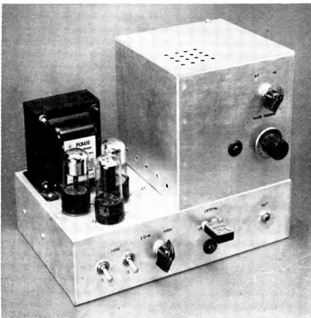
Fig. 6-46 — Pictured is the completed 6146 rig. The plate-current indicator lamp is to the left of the tuning knob. In areas where TVI is likely to be a problem, a metal bottom plate should be used on the chassis in addition to the 6 \times 6 \times 6 aluminum box shown.
