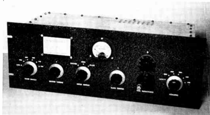
Fig. 6-59 — Controls, from left to right, are for band switch, exciter tuning, meter switch, pi-section tank capacitor, rotary inductor and turns counter, and output-capacitor switch. The panel is 7 by 19 inches. The top cover (a chassis bottom cover) is in place in this view.
