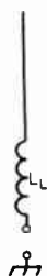
Fig. 19-34 — The capacitive reactance at frequencies lower than the resonant frequency of the whip can be canceled out by adding an equivalent inductive reactance in the form of a loading coil in series with the antenna.
