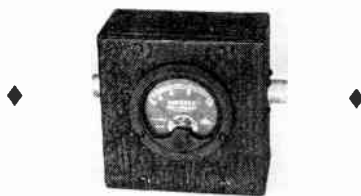
Fig. 21-29 — R.f. ammeter mounted for connecting into a coaxial line for measuring power. A "2-inch" instrument will fit into a 2 \times 4 \times 4 metal box. The shunt capacitance of an ammeter mounted in this way has a negligible effect on the accuracy at frequencies as high as 30 Mc. if the instrument has a bakelite case. Metal-cased meters should be mounted on a bakelite panel which can in turn be mounted in a cut-out which clears the meter case by about \frac{1}{4} inch.
