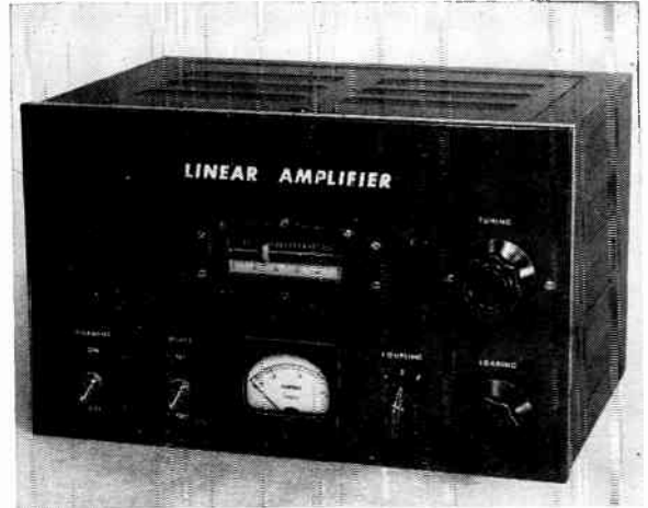
Fig. 12-18 — This linear amplifier uses four parallel-connected tetrodes in a grounded-grid circuit. It can be driven by an s.s.b. exciter capable of 20 watts peak envelope power output. The cabinet is 14½ by 9 by 10 inches deep.
