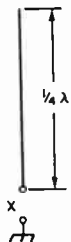
Fig. 19-32 — The quarter-wave whip at resonance will show a pure resistance at the feed point X.
