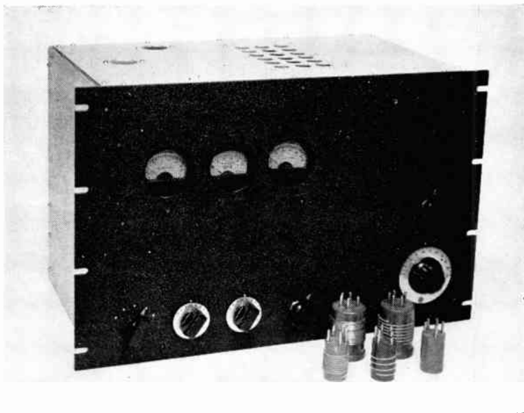
◆ Fig. 6-77 — The panel of the 813 transmitter is 12\frac{1}{4} inches high. The meters are sub-mounted on a piece of \frac{1}{4} -inch Presdwood, 9\frac{1}{2} by 2\frac{7}{8} inches and the openings are covered with a piece of screening. The controls for C_{15} and the link-coupling adjustment are to the right. ◆
