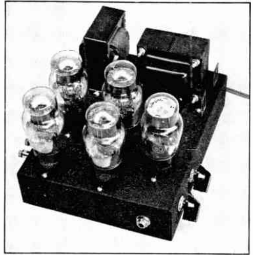
Fig. 8-10 — A vacuum-tube keyer, built up on a 7 \times 9 \times 2 -inch chassis with space for four or less keyer tubes and the power-supply rectifier. The resistors and condensers that produce the lag are underneath, controlled by the knobs at the right. The jack is for the key, while terminals at the left are for the keyed circuit.
