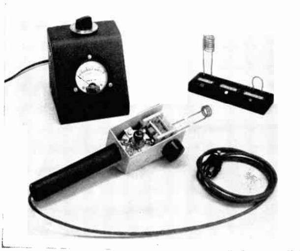
Fig. 21-24 — V.H.F. regenerative wavemeter/grid-dip meter, covering the 50–250 Mc. range. This is a high-sensitivity absorption-type wavemeter particularly useful for checking transmitter harmonics in television bands. The case in which the meter is mounted also contains the power supply. Regeneration is controlled by the knob on top of the case.
