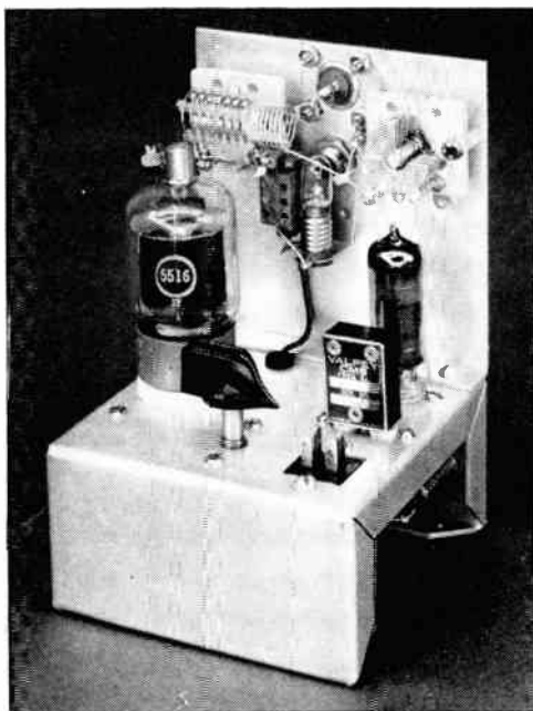
Fig. 20-22 — Rear view of the 50-Mc. r.f. section. The knob above the chassis is the cathode control. The final tank circuit is at the upper left, with antenna series tuning at the upper right.
