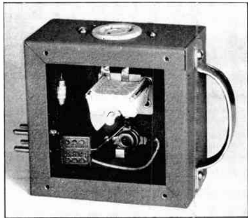
Fig. 21-11 — A rear view of the absorption-type frequency meter. The crystal is wired between the connector plug at the left and the coil socket at the top. The meter by-pass condenser is mounted between the plug and the grounded side of the 'phone jack. The variable-condenser terminals are connected directly to the coil socket.
