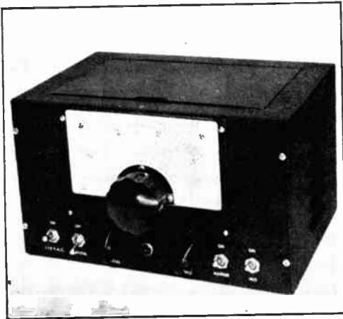
Fig. 21-3 — Additive frequency meter with self-contained power supply. The small knobs are for correction of drift so that both the 100-ke. crystal oscillator and VFO can be set to exact frequency. Dial calibration is in 1000-cycle intervals. This unit can be used for high-accuracy frequency measurement at all frequencies from 100 kc. through 30 Mc.
