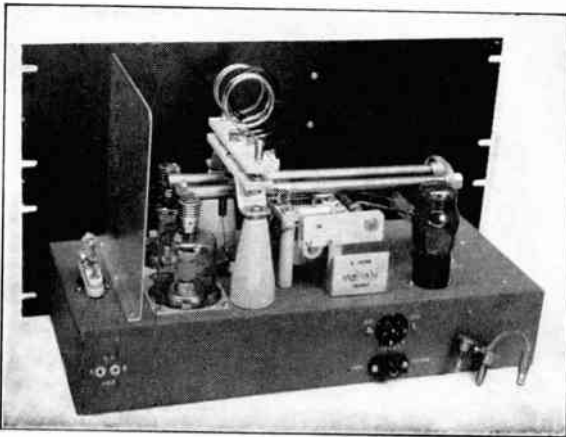
Fig. 17-11 — Rear view of the 4-65A amplifier, showing the two-band tank circuit set up for 50-Mc. operation. R.f. input terminals are on the rear wall to the left and receptacles for the power leads are to the right. The 144-Mc. output terminals are on a bracket to the left of the protective tube. The 50-Mc. output terminal is mounted directly on the XB-15 socket for the plate coil. A plug-in shorting bar, used across the plate lines at 144 Mc., is shown in the foreground.
