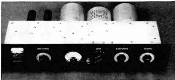
Fig. 6-57 — A compact and completely shielded low-power transmitter using a 6146 as the final amplifier. It can be used at an input of 90 watts on c.w. or 67 watts for plate-modulated 'phone. The unit is mounted on a 3½-inch rack panel.
