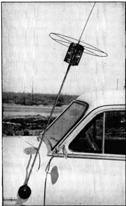
Fig. 20-33 — The top-loaded 4-Mc. antenna used by W6SCN. The loading coil is a B & W transmitting coil. The coil can be tuned by the variable link which is connected in series with the two halves of the coil.
