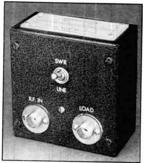
Fig. 21-54 — The coax connectors and voltmeter switch are operated from the rear of the s.w.r. bridge. Care should be taken to remove paint from the panel underneath the connectors. The opposite side of the instrument contains only the indicating meter, which is connected to the switch with flexible leads of sufficient length to permit easy removal of either side.
