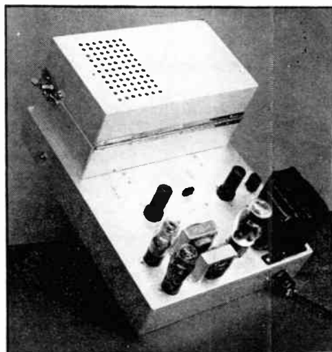
Fig. 6-54 — Rear view, showing the placement of the exciter tubes and the shorting-plug sockets.
