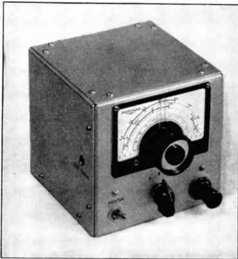
Fig. 20-7 — A bandswitching converter for 6, 10 and 11 meters. The pilot light at the lower right has an adjustable beam, for convenience in mobile work.
