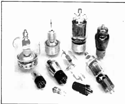
Representative tube types. The miniature, metal-envelope and small glass tubes in the foreground are receiving types. The two tubes with connections at the top of the bulb, lying down, are transmitting triodes of moderate power ratings. Those in the rear are transmitting-type beam tetrodes.
