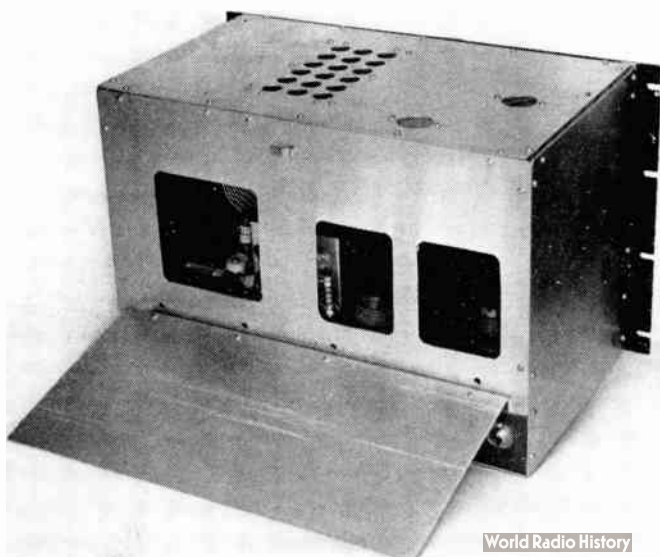
Fig. 6-82 — The shielding enclosure for the 813 transmitter is made up of aluminum sheets fastened together with strips of angle stock, which are tapped for the screws. A hinged door covers the holes that provide access to the plug-in coils. The large opening to the left is 1 1/4 inches square, the other two are 3 by 4 inches. The ventilating holes over the tubes are covered underneath with screening. The back panel is also cut out to clear the terminals set in the rear of the chassis, as shown in Fig. 6-79.
