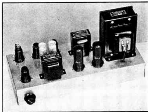
FIG. 1204 — METAL-TUBE SPEECH UNIT WITH PUSH-PULL 6L6 OUTPUT
