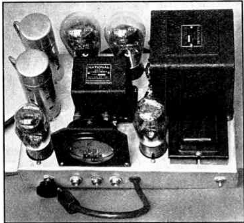
FIG. 1207 — THE ECONOMY MODULATOR UNIT CONTAINS A CRYSTAL-MICROPHONE SPEECH AMPLIFIER, DRIVER AND CLASS-B MODULATOR, AS WELL AS A POWER SUPPLY FOR THE LOW-POWER STAGES
