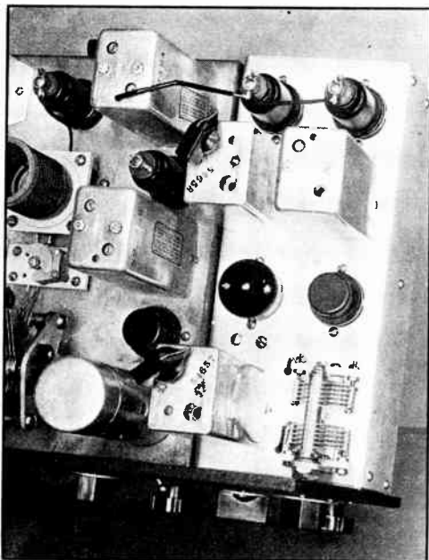
FIG. 727 — THE CRYSTAL FILTER AND NOISE-SILENCER UNIT ATTACHED TO THE HIGH-PERFORMANCE SUPER
