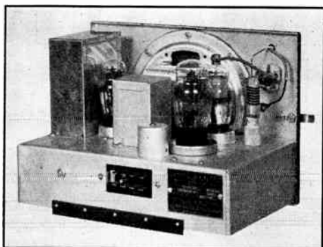
FIG. 1312—A MOBILE RECEIVER EMPLOYING THE CIRCUIT GIVEN IN FIG. 1311 The tube shields have been removed.
