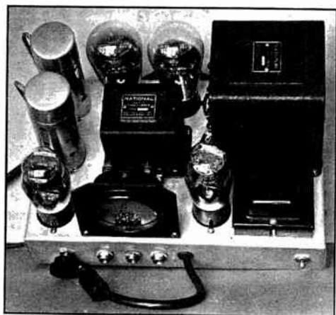
FIG. 1203 — THE ECONOMY MODULATOR UNIT CONTAINS A CRYSTAL-MICROPHONE SPEECH AMPLIFIER, DRIVER AND CLASS-B MODULATOR, AS WELL AS A POWER SUPPLY FOR THE LOW-POWER STAGES
