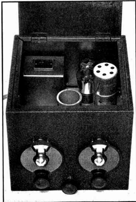
FIG. 702—THIS TWO-TUBE RECEIVER HAS A CONTINUOUS FREQUENCY RANGE OF 1450 TO 41,000 KILOCYCLES AND GIVES COMPLETE BAND-SPREAD ON FIVE AMATEUR BANDS
