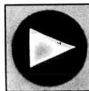
FIG. 1213-G — ACTUAL PHOTOGRAPH OF TRAPEZOIDAL FIGURE FOR PROPER 100% MODULATION
