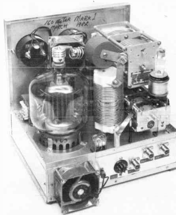
Fig. 58 — Rear view of the 160-meter amplifier with the cover removed. The chassis dimensions are 10 × 12 × 13 inches. Seen here are the plate-circuit components. K1 is the small relay at the rear of the chassis. The large cylindrical object above the tank inductor is the plate-blocking capacitor. Between the tuning and loading capacitors is a 220-pF vacuum capacitor to supplement the variable unit. The loading capacitor is a 5-gang assembly. Behind the tube from left to right are T1, T2 and RFC2. Directly behind the anode cap and parasitic choke is the upper fan.
