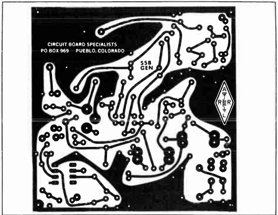
Fig. 43 — Full-scale etching pattern for the ssb generator pc board, shown from the foil side. Black represents unetched copper.
