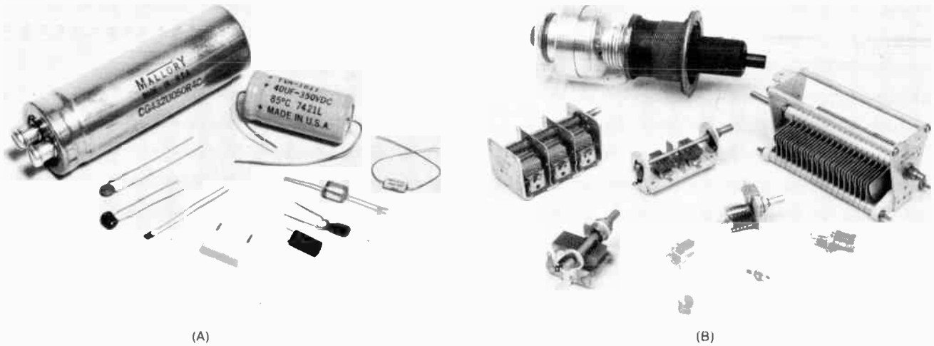
Fig. 15 — Fixed-value capacitors are shown at A. A large computer-grade unit is at the upper left. The 40- \mu F unit is an electrolytic capacitor. The smaller pieces are silver-mica, disc-ceramic, tantalum, polystyrene and ceramic chip capacitors. The small black unit (cylindrical) is a pc-board-mount electrolytic. Variable capacitors are shown at B. A vacuum variable is at the upper left.
