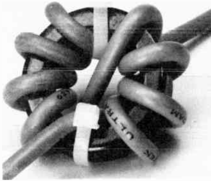
Fig. 6 — Winding the cable on a ferrite toroid is a highly effective shield current suppressor in some cases. Reversing the winding as pictured allows more turns with less shunt capacitance. RG-58 will suffice for moderate power applications. The most important property of the cable is complete shielding — avoid "bargain" cable having less than 95-percent braid coverage.
