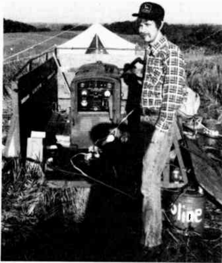
Fig. 13 — Large gasoline generators of the kW and higher class are excellent for powering several amateur stations from a complex field site. Maintenance, as discussed in the text, is a vital matter to ensure reliable operation. Here, WB9QPI has just finished a maintenance check of the group's Field Day power plant.
