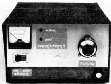
Fig. 21 — A 500-watt amplifier for the 2-meter band, complete with power supply, is housed in this cabinet. The hole plug covers a former location of a control.
