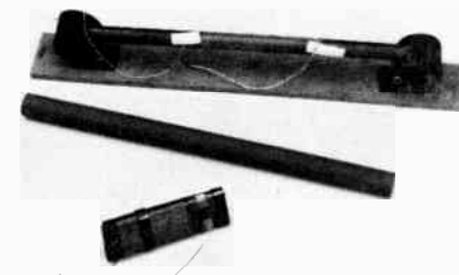
Fig. 52 — A bc-band ferrite rod loop antenna is at the top of the picture (J.W. Miller Co.). A blank ferrite rod is seen at the center and a flat bc-band ferrite loop antenna is in the lower foreground.
