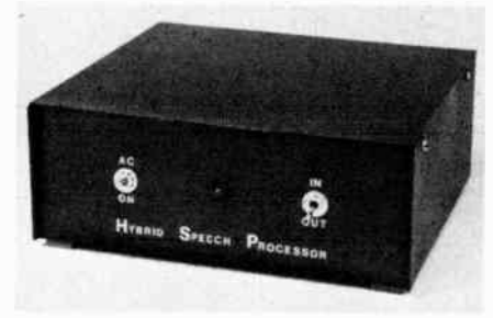
Fig. 35 — Exterior view of the outboard speech processor. The lack of external adjustments makes the unit easy to use and difficult to abuse.
