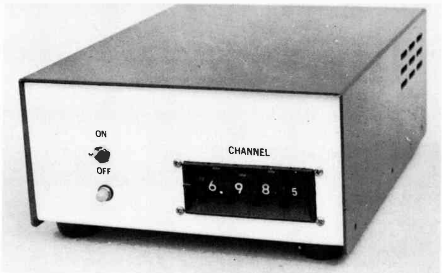
Fig. 24 — Front panel on the synthesized 2-meter transmitter showing the ON-OFF switch and the frequency-selector switches. The microphone connector and accessory jack are located on the rear panel.
