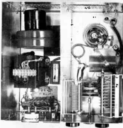
Fig. 77 — Top view of the 3-500Z amplifier. The top section of the amplifier is divided into two compartments. One contains the power supply and blower and the other holds the rf components.
