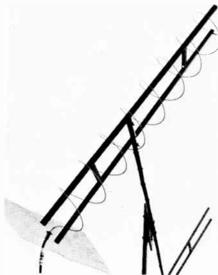
Fig. 17 — An eight-turn 432-MHz helical array, wound from aluminum clothesline wire. Left-hand polarization is shown. Each turn is one wavelength, with a pitch of 0.25 wavelength. Feed is with 50-ohm coax, through an 84-ohm Q section.
