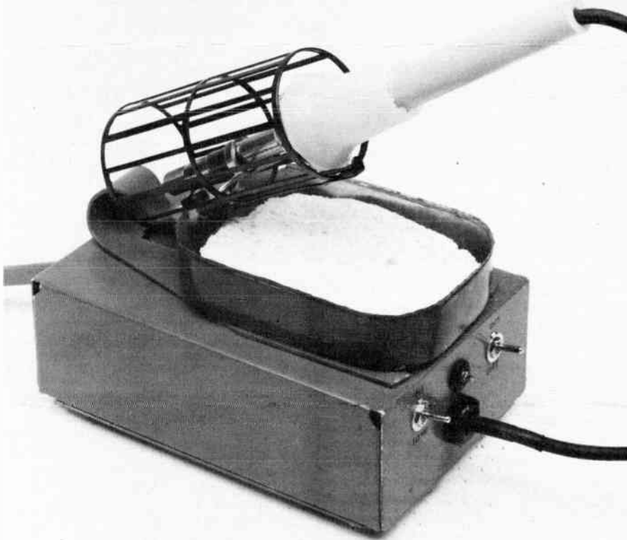
Fig. 1 — A compact assembly of commonly available items, this soldering station sanitizes the electronics assembly process. Miniature toggle switches are used because of the minimal force required to manipulate them. The force required to operate standard-size switches could destabilize the unit.
