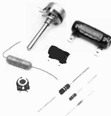
Fig. 7 — Examples of various resistors. In the foreground are 1/4-, 1/2- and 1-watt composition resistors. The three larger cylindrical components at the center are wirewound power resistors. The remaining two parts are variable resistors, pc-board mount at the lower left and panel mount at the upper center.
