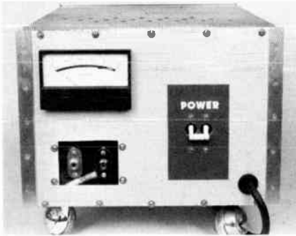
Fig. 51 — Front view of the heavy-duty, 3400-volt power supply.
