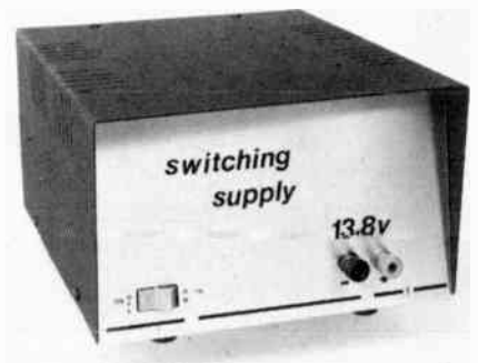
Fig. 46 — Front panel of the switching power supply. The cabinet is by Apollo and has a built-in power switch.
