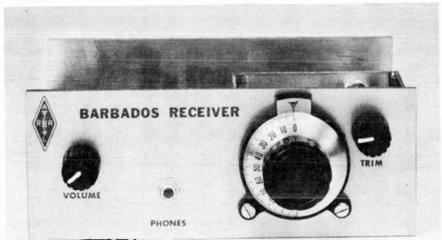
Fig. 55 — A low-cost cw receiver designed by Doug DeMaw, W1FB. The name on the front panel was inspired by the unit's intended purpose — vacation operating.
