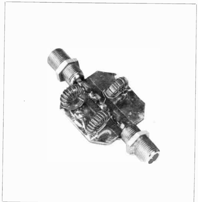
Fig. 21 — Photo showing construction of the 75-ohm unbalanced filter.
