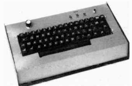
Fig. 20 — The completed Morse keyboard measures 14-1/2 x 8-1/4 x 3-1/4 inches.
