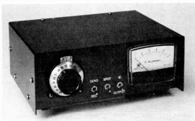
Fig. 49 — Photographs of the completed 6-watt, VXO-controlled transmitter. Miniature coaxial cable (RG-174/U) is used for connections between the circuit board, connectors and switches for all runs carrying rf energy.
