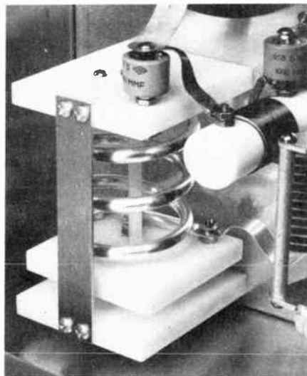
Fig. 16 — Photograph of the assembled adjustable inductor. Make certain to use only plated brass hardware for pieces that come into contact with the coil.
