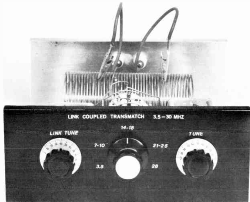
Fig. 26 — Exterior view of the band-switched link coupler. Alligator clips are used to select the proper tap positions of the coil.
