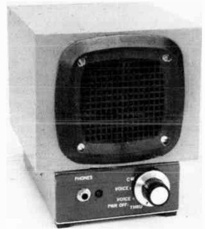
Fig. 84 — Deluxe audio filter with self-contained loudspeaker, built in the ARRL lab by Greg Bonaguide, WA1VUG. The 4-inch speaker is mounted in an enclosure having outside dimensions of 5-1/2 x 6-1/2 x 6-3/4 inches (H x W x D). The chassis measures 2 x 5 x 7 inches.
