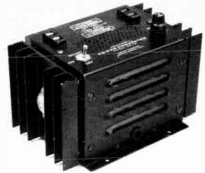
Fig. 12 — Photograph of a commercial dc-to-ac inverter that operates from 6 to 12 volts dc and delivers 117 volts ac (square wave) at 175 watts.
