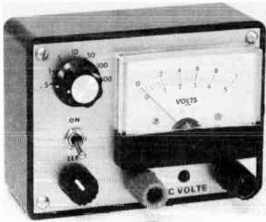
Fig. 9 — The IC voltmeter mounted in a small plastic case. This basic instrument measures only dc voltages, but with an rf probe as described later in this chapter, it can be used for rf measurements as well. It may also be used for resistance measurements, by using techniques described in the previous section. DS1, mounted between the binding posts, is a power-on indicator.
