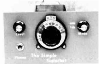
Fig. 63 — Outside view of the simple superhet receiver. The front and rear panels are made from double-sided circuit board.
