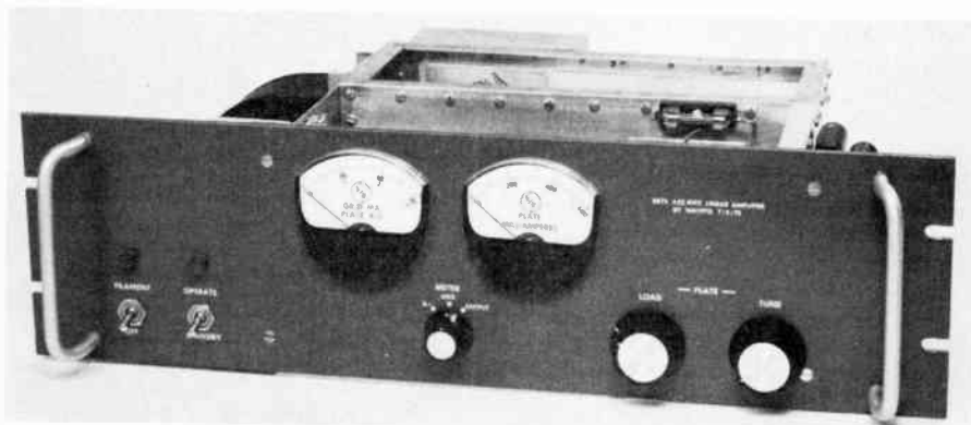
Fig. 35 — The high-power uhf amplifier. The toggle switches control filament power and standby/operate functions respectively. Multimeter function is selected with the switch located between the meters, while the plate tuning and loading controls are at the right. Modern knobs and homemade meter faces give the amplifier a commercial appearance.
