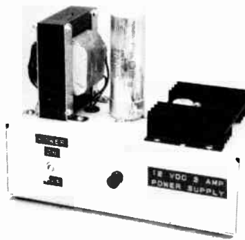
Fig. 31 — Exterior view of the 12-volt, 3-ampere, no-frills power supply.
