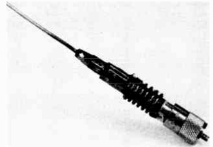
Fig. 24 — Photograph of the 220-MHz 5/8-wavelength mobile antenna. The bottom end of the coil is soldered to the coaxial connector.
