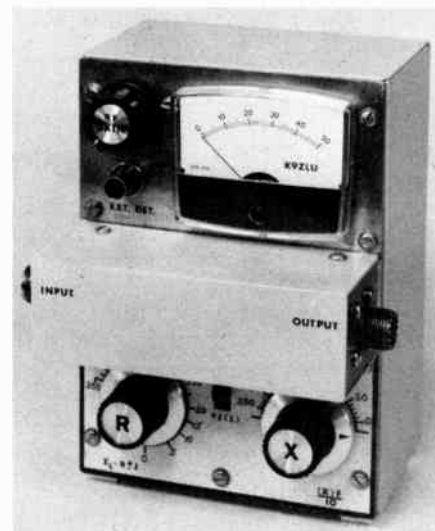
Fig. 73 — The OIB is enclosed in a 7 × 5 × 3-in. (178 × 127 × 76-mm) aluminum chassis. Tinnerman Speed Nuts and machine screws are used to secure the front panel to the chassis flange. Rectangular holes with cover plates in the rear panel permit alignment of the unit while it is fastened to the chassis.
