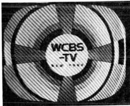
Fig. 2 — "Cross-hatching," caused by the beat between the picture carrier and an interfering signal inside the TV channel.
