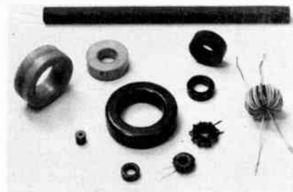
Fig. 50 — An assortment of toroid cores. A ferrite rod is placed at the top of the picture for comparison. The two light-colored, plastic-encased toroids at the upper left are tapewound types (Hypersil steel) are suitable for audio and dc-to-dc converter transformers. The wound toroid at the right center contains two toroid cores which have been stacked atop one another to increase the power capability.
