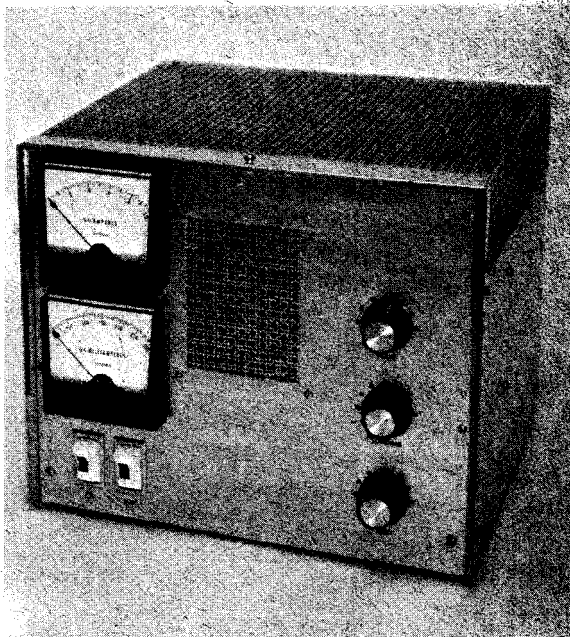
Fig. 7-27 — Table-top 50-MHz amplifier of grounded-grid design, only 10 X 12 inches in size. Grid and plate current are monitored simultaneously. Knobs at the right are for input tuning, bottom, amplifier loading, center, and plate tuning, top.
