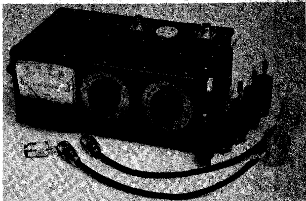
Fig. 1 — An RCL bridge for measuring unknown values of complex impedances. A plug-in coil is used for each frequency band. The bridge operates at an rf input level of about 5 volts; pickup-link assemblies for use with a grid-dip oscillator are shown. Before measurements are made, the bridge must be balanced with a nonreactive load connected at its measurement terminals. This load consists of a resistor mounted inside a coaxial plug, shown in front of the instrument at the left. The aluminum box measures 4 1/4 X 10 3/4 X 6 1/8 inches and is fitted with a carrying handle on the left end and self-sticking rubber feet on the right end and bottom. Dials are Millen No. 10009 with skirts reversed and calibrations added.
