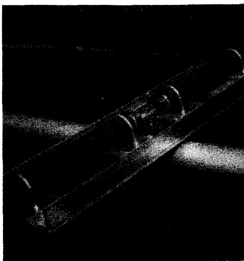
Fig. 3 — The driven element needs to be insulated from the boom. Insulation is provided by PVC tubing held in place on sheet plastic with U bolts.
