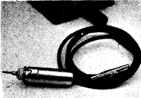
Fig. 17-52 — Rf probe for use with an electronic voltmeter. The case of the probe is constructed from a 7-pin ceramic tube socket and a 2 1/4-inch tube shield. A half-inch grommet at the top of the tube shield prevents the output lead from chafing. A flexible copper-braid grounding lead and alligator clip provide a low-inductance return path from the test circuit.
