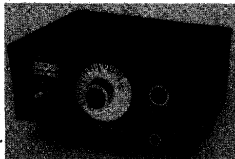
Fig. 3 — Front view of the direct-conversion receiver. The cabinet is homemade from two U-shaped pieces of .040-inch thick sheet aluminum. The front panel is painted battleship gray, and white "press-on" labels mark the function of the controls.
