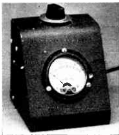
Fig. 21-23 — Power supply and milliammeter for the grid-dip meter are contained in a meter case. The control on top is for varying the plate voltage to maintain the grid current in the proper region.
