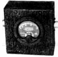
Fig. 21-33 — R.f. ammeter mounted for connecting into a coaxial line for measuring power. A “2-inch” instrument will fit into a 2 × 4 × 4 metal box. The shunt capacitance of an ammeter mounted in this way has a negligible effect on the accuracy at frequencies as high as 30 Mc. if the instrument has a bakelite case. Metal-cased meters should be mounted on a bakelite panel which can in turn be mounted in a cut-out which clears the meter case by about ¼ inch.
