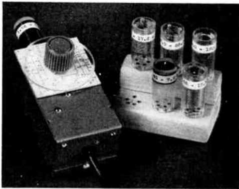
Fig. 21-20 — A compact and light-weight grid-dip meter for one-hand operation. It is built in a 1 3/4 x 2 1/2 x 1-inch "Channel-lock" box and uses six plug-in coils to cover the range 1600 kc. to 160 Mc. The power supply and milliammeter for reading grid current are in a separate unit.
