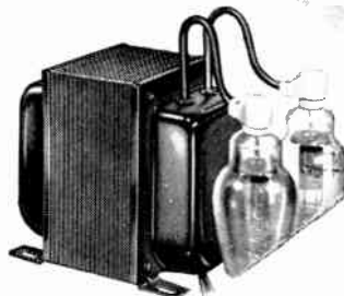
PLATE TRANSFORMER, PT8315 . Mounting style provides protected path to anodes of rectifier tubes with heavily insulated HV leads out of top of unit. Primary leads brought out through bottom. Primary, 117 volts, 60 cycles; secondary, 2065-0-2065 AC volts; 1750 DC volts, DCMA 200 CCS, 250 ICAS, weight 24 pounds. DC output rated at load terminals of single-section, reactor-input filter with full-wave mercury vapor rectifiers.
