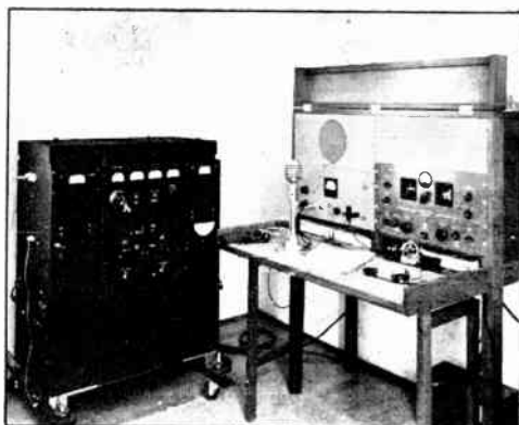
In this example of a compact high-power station, the operating table folds up when not in use and covers the receiver and speech amplifier. Special furniture, like this homemade operating table, goes a long way toward solving the space problem for many amateurs. (W4HAY, Fort Thomas, Ky.)
