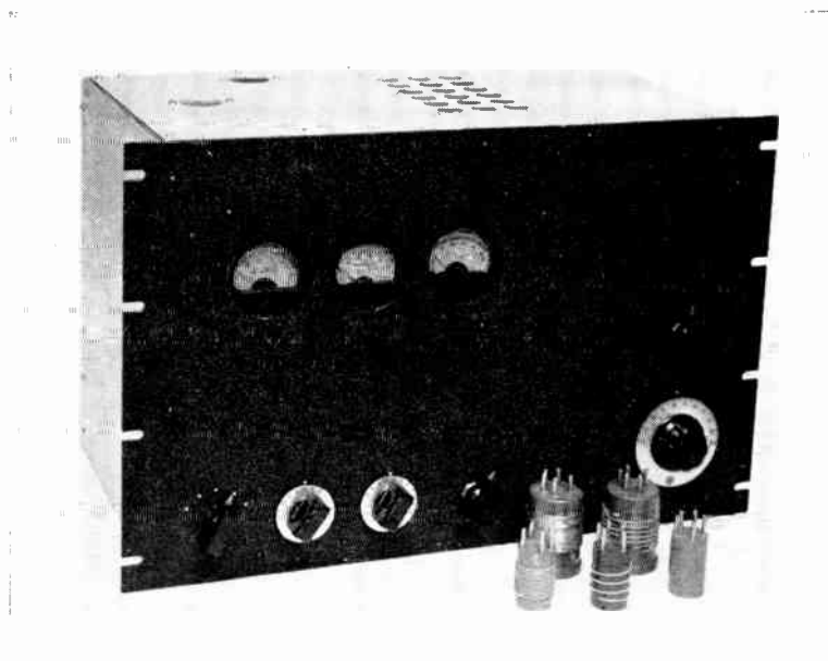
Fig. 6-70 — The panel of the 813 transmitter is 12\frac{1}{4} inches high. The meters are sub-mounted on a piece of \frac{1}{4} -inch Pres-dwood, 9\frac{1}{2} by 27.8 inches and the openings are covered with a piece of screening. The controls for C_{13} and the link-coupling adjustment are to the right.
