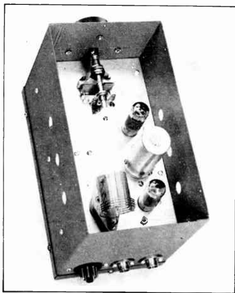
Fig. 6-83 — The top of the simple VFO showing the oscillator tuning condenser, the tubes and plug-in coils.
