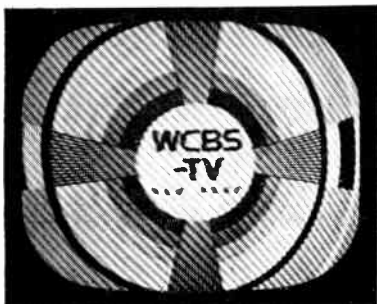
Fig. 23-8 — "Crosshatching," caused by the beat between the picture carrier and an interfering harmonic inside the TV channel.
