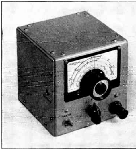
Fig. 20-10 — A handswitching converter for 6, 10 and 11 meters. The pilot light at the lower right has an adjustable beam, for convenience in mobile work.
