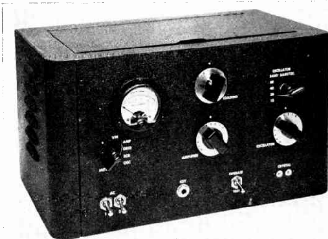
Fig. 6-54 — The complete 75-watt 6-band transmitter fits into an 8 × 11 × 8-inch cabinet. Along the bottom, from left to right, are the two power switches ( S_5 and S_6 ), the key jack ( J_7 ), the "operate-test" switch ( S_4 ) and the crystal socket. Across the center are the meter switch ( S_3 ), the amplifier tank control ( C_9 ) and the oscillator tuning condenser ( C_8 ). To the right of the meter at the top are the loading condenser ( C_{10} ) and the oscillator bandswitch ( S_2 ).
