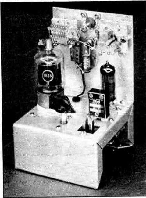
Fig. 20-21 — Rear view of the 50-Mc. r.f. section. The knob above the chassis is the cathode control. The final tank circuit is at the upper left, with antenna series tuning at the upper right.
