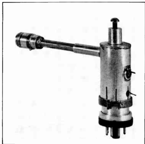
Fig. 19-23 — A half-wave cavity oscillator for 2300 Mc. (W2RMA)
