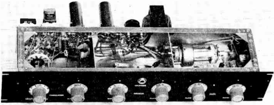
Fig. 17-8 — Looking into the handswitching exciter-transmitter from the top front. Oscillator components are in the left compartment, the doubler and power connector in the center, and the output stage at the right. Note that the 6L16 socket is mounted inside the output stage compartment.
