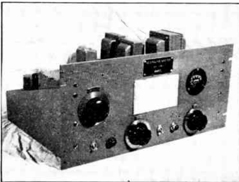
Fig. 6-92 — A beat-frequency exciter built by W6RZL. The dial at the left controls the frequency of the VFO and thereby the frequency of the exciter output. The other two dials are for the crystal-oscillator and amplifier-output tanks.
