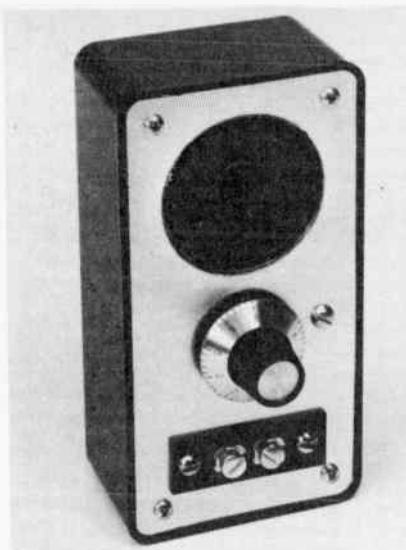
A code practice oscillator that can be constructed from commonly available parts.
