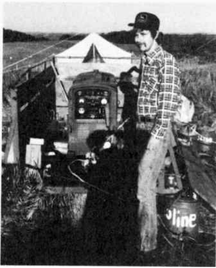
Fig. 13 — Large gasoline generators of the kW and higher class are excellent for powering several amateur stations from a complex field site. Maintenance, as discussed in the text, is a vital matter to ensure reliable operation. Here, WB9QPI has just finished a maintenance check of the group's Field Day power plant.
