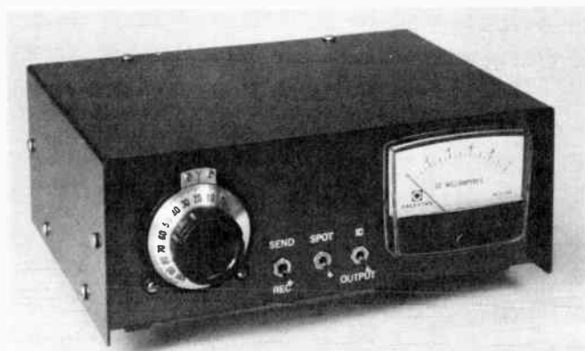
Fig. 49 — Photographs of the completed 6-watt, VXO-controlled transmitter. Miniature coaxial cable (RG-174/U) is used for connections between the circuit board, connectors and switches for all runs carrying rf energy.
