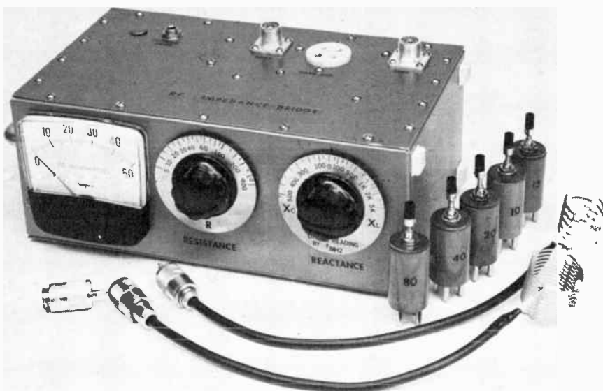
Fig. 60 — An RCL bridge for measuring unknown values of complex impedances. A plug-in coil is used for each frequency band. The bridge operates at an rf input level of about 5 volts; pickup-link assemblies for use with a grid-dip oscillator are shown. Before measurements are made, the bridge must be balanced with a nonreactive load connected at its measurement terminals. This load consists of a resistor mounted inside a coxial plug, shown in front of the instrument at the left. The aluminum box measures 4-1/4 x 10-3/4 x 6-1/8 inches (108 x 273 x 156 mm) and is fitted with a carrying handle on the left end and self-sticking rubber feet on the right end and bottom. Dials are Millen no. 10009 with skirts reversed and calibrations added.
