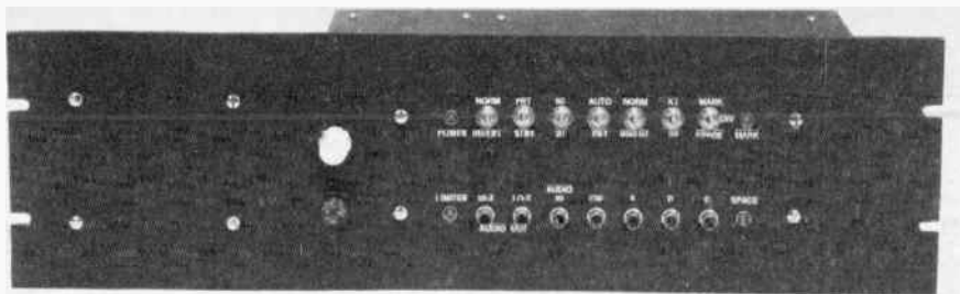
Fig. 60 — This RTTY terminal unit can be used with any combination of equipment. It was built by Ed Kalin, K1RT, in the ARRL laboratory. Circuit design is by W1RN.
