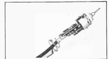
Fig. 20 — Inside the probe. The 1N34A diode, calibrating resistor and input capacitor are mounted tight to the terminal strip with shortest leads possible. Spaghetti tubing is placed on the diode leads to prevent accidental short circuits. The tube-shield spring and flexible-copper grounding lead are soldered to the cable braid (the cable is RG-58/U coax). The tip can be either a phone tip or a short pointed piece of heavy wire.
