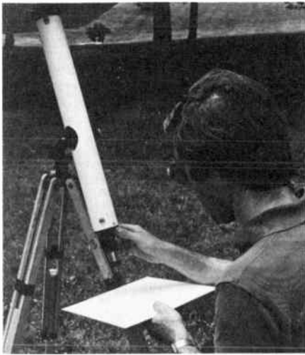
Fig. 2 — A simple sunspot projection system, demonstrated by ARRL staffer AC1Y. The card-board baffle at the top provides a shaded area for viewing the sun's image. Never look at the sun with the naked eye, binoculars or telescope, except through a known safe solar filter. See page 18-9 for additional cautions.
