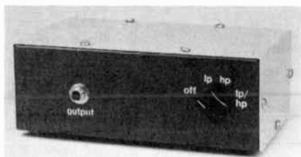
Fig. 89 — Photograph of the space-perception cw filter. Press-on lettering was used to label the control and jack functions.
