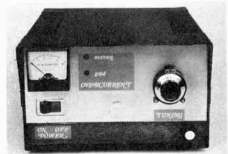
Fig. 21 — A 500-watt amplifier for the 2-meter band, complete with power supply, is housed in this cabinet. The hole plug covers a former location of a control.
