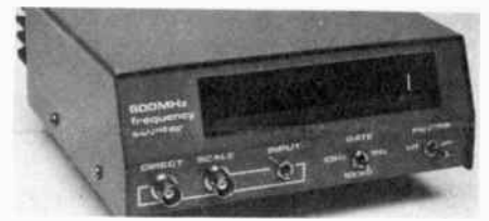
Fig. 30 — Exterior view of the 600-MHz frequency counter. The last digit is not blanked in order to provide an on-off indicator.
