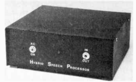
Fig. 35 — Exterior view of the outboard speech processor. The lack of external adjustments makes the unit easy to use and difficult to abuse.
