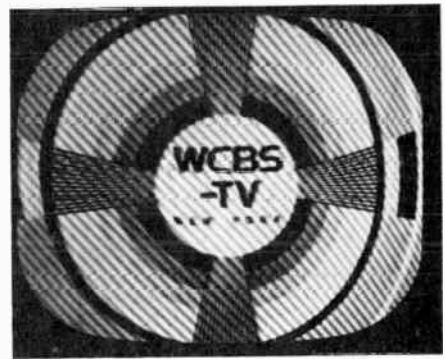
Fig. 3 — "Cross-hatching," caused by the beat between the picture carrier and an interfering signal inside the TV channel.
