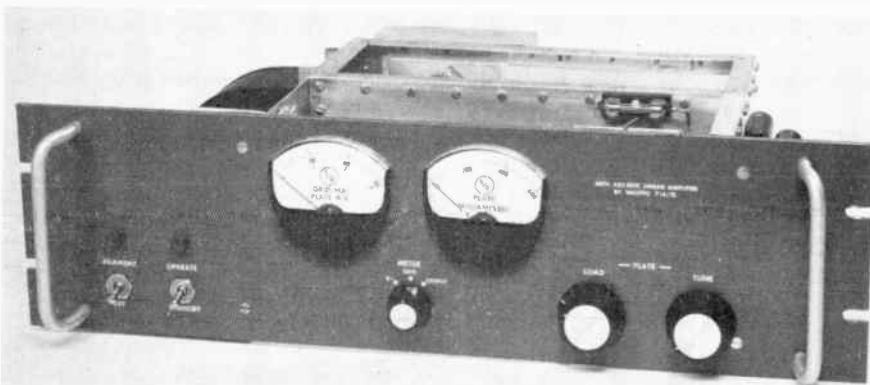
Fig. 35 — The high-power uhf amplifier. The toggle switches control filament power and standby/operate functions respectively. Multimeter function is selected with the switch located between the meters, while the plate tuning and loading controls are at the right. Modern knobs and homemade meter faces give the amplifier a commercial appearance.
