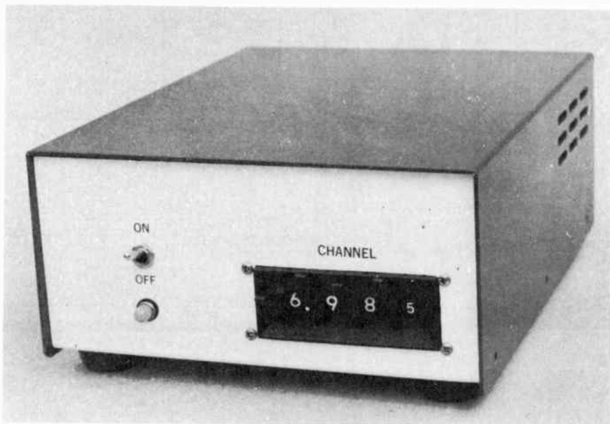
Fig. 24 — Front panel on the synthesized 2-meter transmitter showing the ON-OFF switch and the frequency-selector switches. The microphone connector and accessory jack are located on the rear panel.
