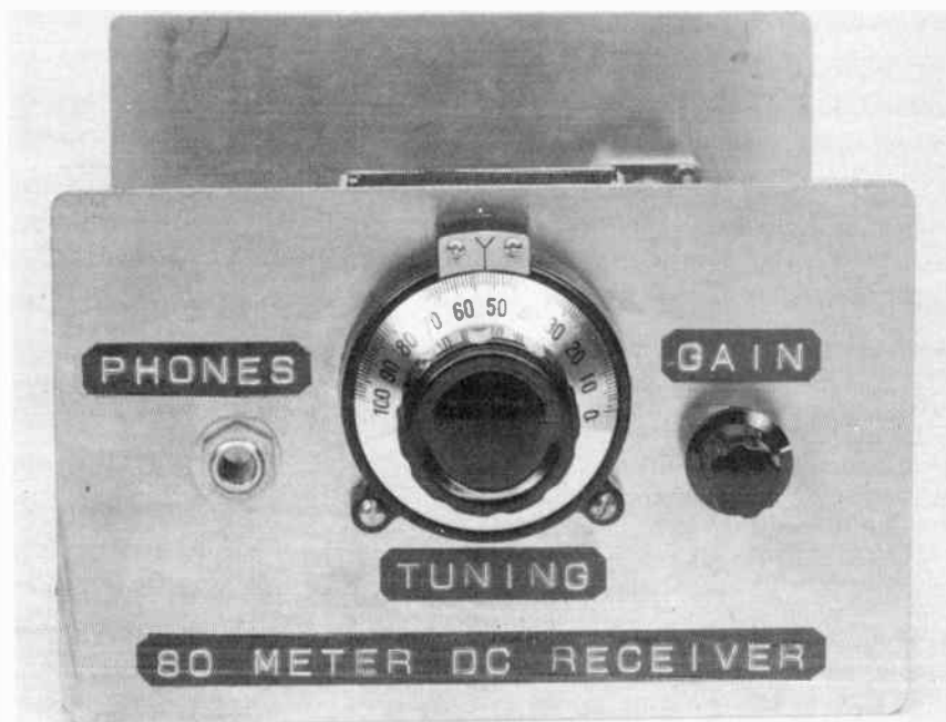
Fig. 55 Front view of the beginner's receiver. The panels are made from double-sided pc board material.
