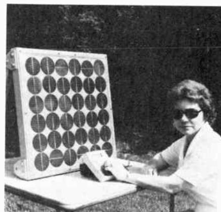
Fig. 9 — Solar-electric arrays are excellent for short-or long-term field and emergency use to power amateur stations. A 14-volt, 1.5-A solar panel and two automobile batteries in parallel can provide many after-dark hours of operation with typical 100-watt hf-band transceivers of the solid-state variety.
