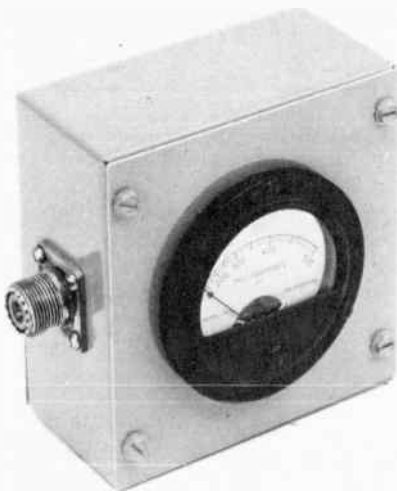
Fig. 13 — Rf ammeter mounted in a Minibox, with connectors for placing the meter in series with a coaxial line. A bakelite-case meter should be used to minimize shunt capacitance (which introduces error) although a metal-case meter can be used if mounted on bakelite sheet with a large cut-out in the case around the rim. The meter can be used for rf power measurements ( P = I^2R ) when connected between the transmitter and a nonreactive load of known resistance.
