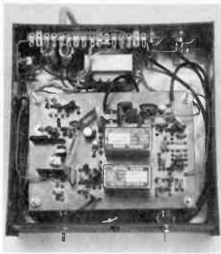
Fig. 39 — Interior view of the speech processor, showing the rf board. The audio board nests beneath the rf board. The power supply components and microphone connectors are mounted on the rear panel.
