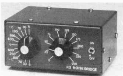
Fig. 68 — Exterior view of the noise bridge. The unit is finished in red enamel. Press-on lettering is used for the calibration marks.
