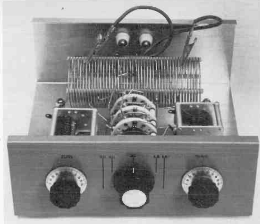
Fig. 27 — Exterior view of the band-switched link coupler. Alligator clips are used to select the proper tap positions of the coil.
