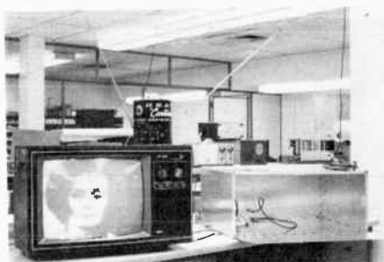
Fig. 7 — Lab simulation of TVI tests discussed in the text. A dummy load placed next to the "rabbit ears" served as the transmitting antenna.
