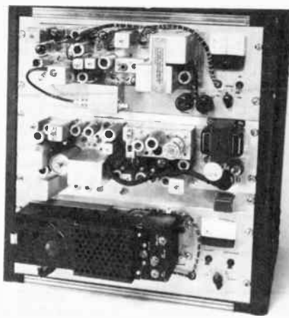
Fig. 39 — This typical 144-MHz amateur repeater uses GE Progress-Line transmitter and receiver decks. Power supplies and metering circuits have been added. The receiver located on the middle deck is a 440-MHz control receiver, also a surplus GE unit. A preamplifier, similar to that shown in Fig. 30, has been added to the 2-meter receiver to improve the sensitivity so that a 0.2- \mu V input signal will produce 20 dB of quieting.
