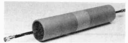
Fig. 10 — This coax shield decoupler is made with steel wool stuffed into an IBM copier tube. This size was selected for photographic purposes, but to be truly effective, the device should be about twice as long.
