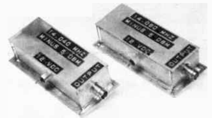
Fig. 81 — Exterior view of the signal generators suitable for use in receiver performance measurements. Each uses an OE-10 oscillator available from International Crystal Mfg. Co., Inc.
