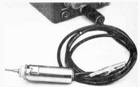
Fig. 18 — Rf probe for use with an electronic voltmeter. The case of the probe is constructed from a seven-pin ceramic tube socket and a 2-1/4-inch (57-mm) tube shield. A half-inch (13-mm) grommet at the top of the tube shield prevents the output lead from chafing. A flexible copper-braid grounding lead and alligator clip provide a low-inductance return path from the test circuit.
