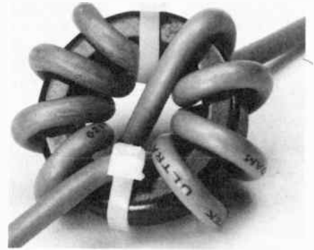
Fig. 11 — Winding the cable on a ferrite toroid is a highly effective shield current suppressor in some cases. Reversing the winding as pictured allows more turns with less shunt capacitance. RG-8X is used in this model, but RG-58 will suffice for moderate power applications. The most important property of the cable is complete shielding — avoid "bargain" cable having less than 95-percent braid coverage.
