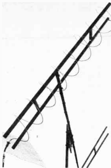
Fig. 17 — An eight-turn 432-MHz helical array, wound from aluminum clothesline wire. Left-hand polarization is shown. Each turn is one wavelength, with a pitch of 0.25 wavelength. Feed is with 50-ohm coax, through an 84-ohm Q section.
