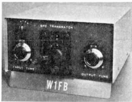
Fig. 22 — Exterior view of the SPC Transmatch. Radio Shack vernier drives are used for adjusting the tuning capacitors. A James Millen turns-counter drive is coupled to the rotary inductor. Green paint and green Dymo tape labels are used for panel decor. The cover is plain aluminum with a lightly grooved finish (sandpapered) which has been coated with clear lacquer. An aluminum foot holds the Transmatch at an easy access angle.
