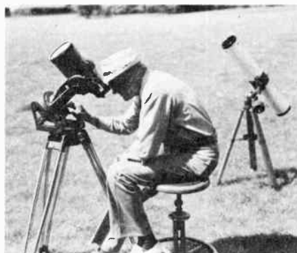
Fig. 8 — Direct viewing of the sun should be done only with a telescope equipped with an aperture filter known to be safe for this purpose. Telescope is a Celestron 5 with the maker's solar filter, which passes 0.01 percent of impinging light. A brimmed hat shading the observer's eyes from direct rays of the sun helps to improve visual acuity.
