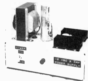
Fig. 31 — Exterior view of the 12-volt, 3-ampere no-frills power supply.
